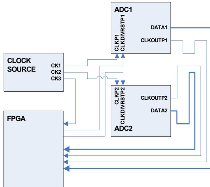
FIGURE 4. MULTIPLE ADC SYNCHRONIZATION CIRCUITRY
