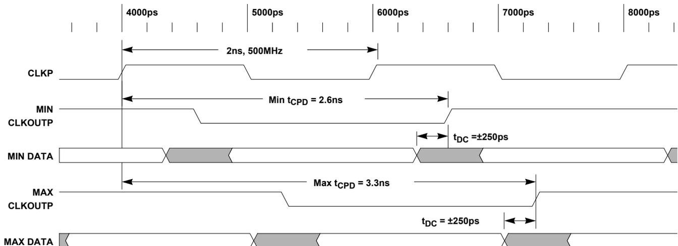
FIGURE 1. 1.8V AT  $+25^\circ\text{C}$  ADC OUTPUT TIMING
