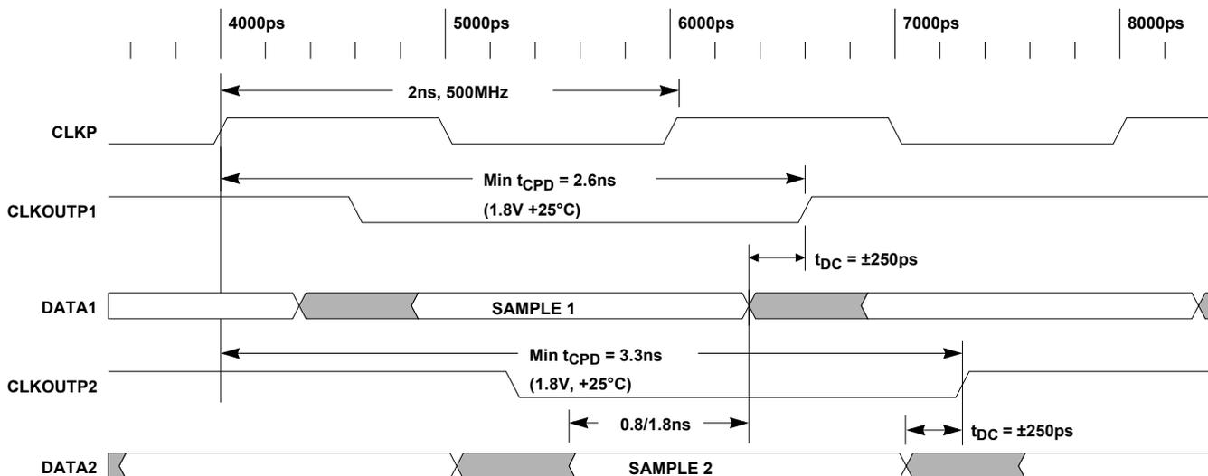
FIGURE 5. 1.8V AT +25°C MULTIPLE ADC TIMING SKEW
