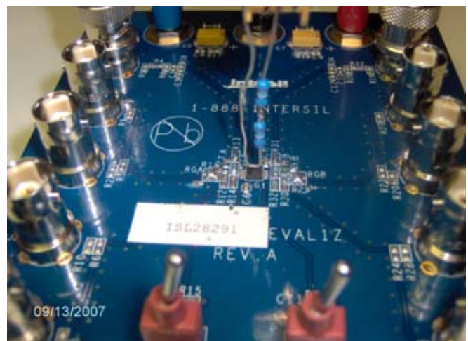
FIGURE 8. IMPROVED ANTENNA DESIGN TO EVALUATE RADIATED INTERFERENCE
