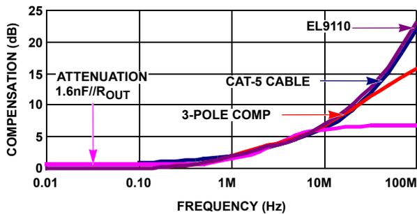
FIGURE 13. 100m CAT-5 CABLE ATTENUATION AND COMPENSATION
