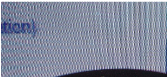
FIGURE 9. EXAMPLE OF LOSS OF HORIZONTAL SYNCHRONIZATION
