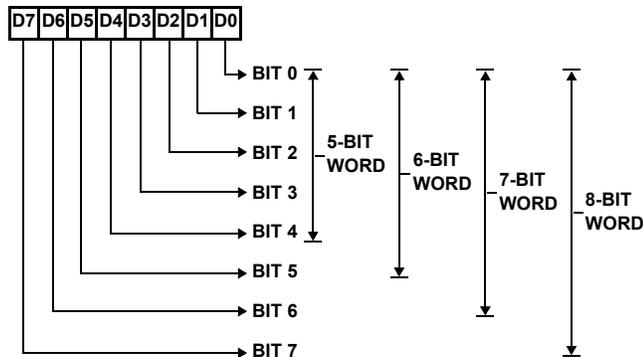
NOTE: THE LSB, BIT 0 IS THE FIRST SERIAL DATA BIT RECEIVED
