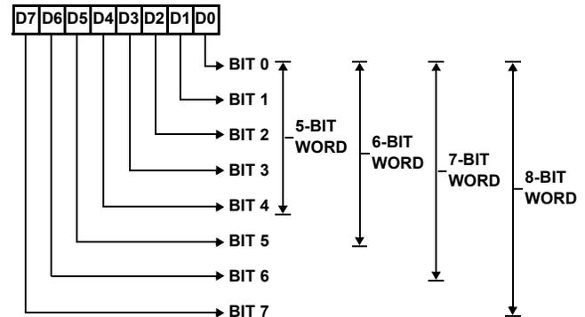
NOTE: THE LSB, BIT 0 IS THE FIRST SERIAL DATA BIT TRANSMITTED
