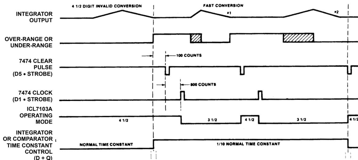
FIGURE 7. TIMING DIAGRAM FOR CIRCUIT #2
