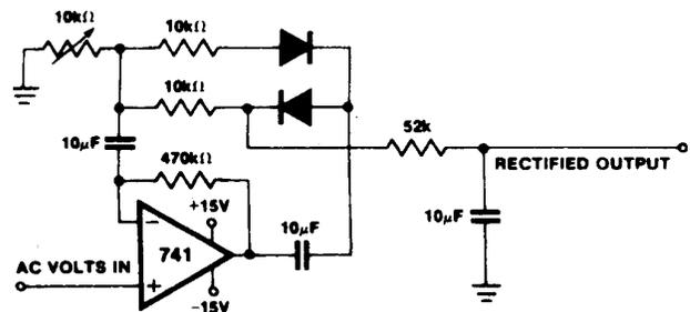
FIGURE 3. PRECISION RECTIFIER AND LOW PASS FILTER
