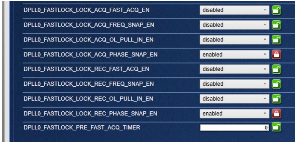
Figure 23. DPLL Channel 0 Fast Lock Register Configuration for Line Card
