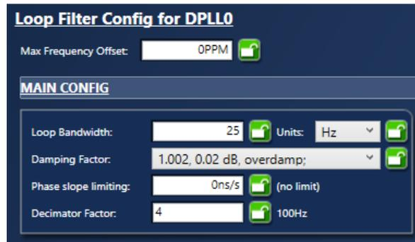
Figure 8. DPLL Channel 0 Loop Filter for Master
