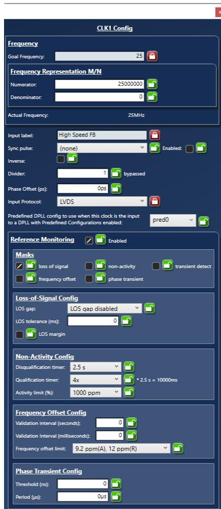
Figure 20. Feedback Input for Line Card
