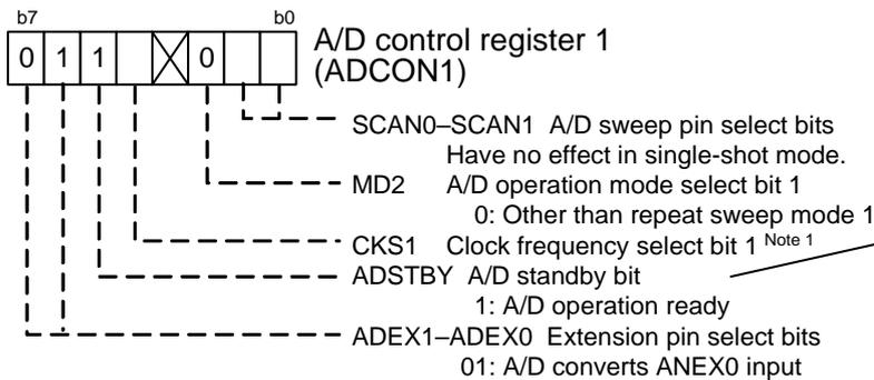
If the ADSTBY bit is changed from 0 (A/D operation stopped) to 1 (A/D operation ready), wait 1  $\phi_{AD}$  cycle or more before starting A/D conversion.
