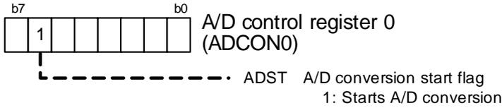
The ADST bit reads 0 when it is read before an A/D conversion starts after writing 1 to the ADST bit.
