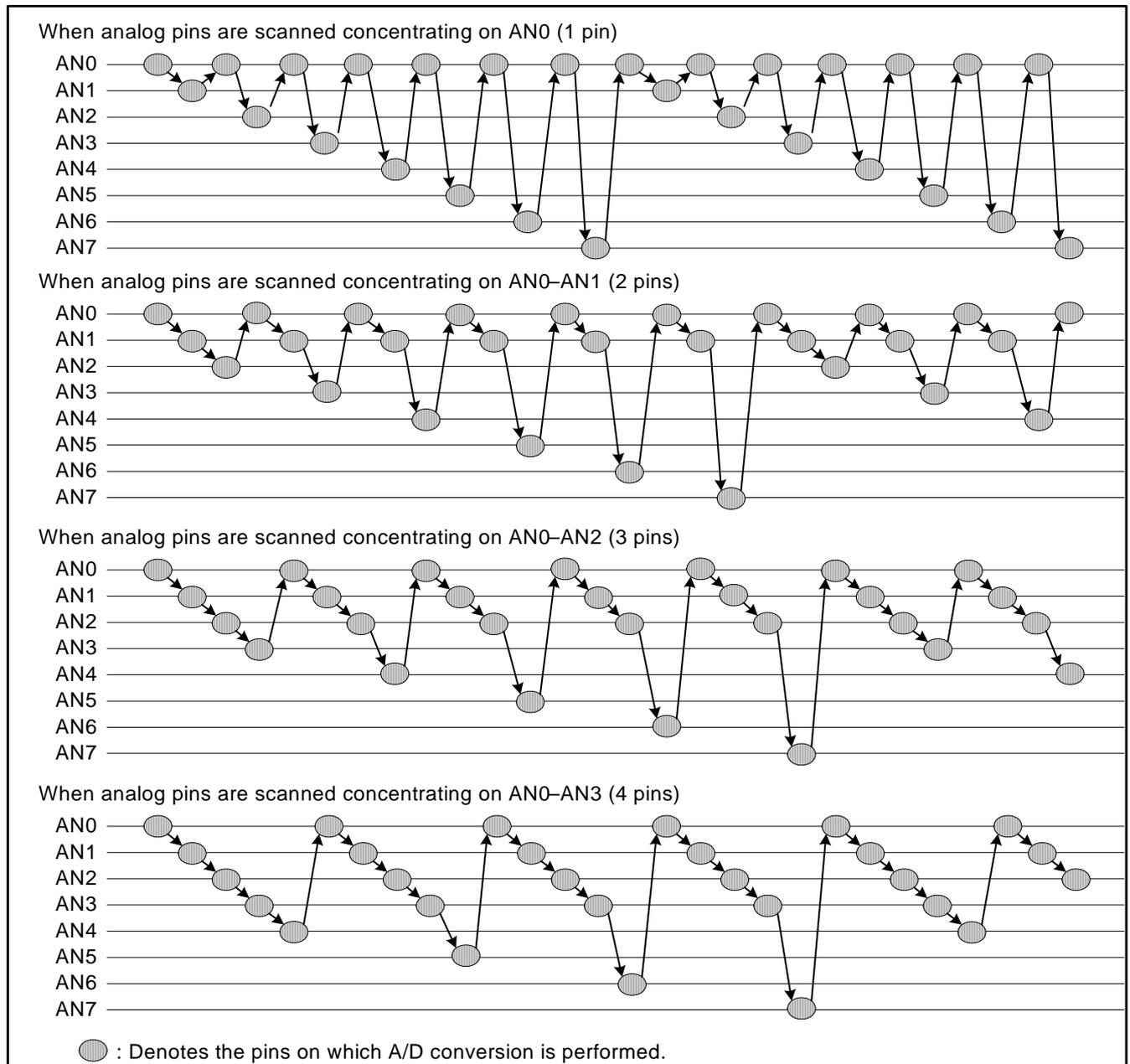
Figure 1. The Order in Which AN0–AN7 Pins are Scanned in Repeated Sweep Mode 1
