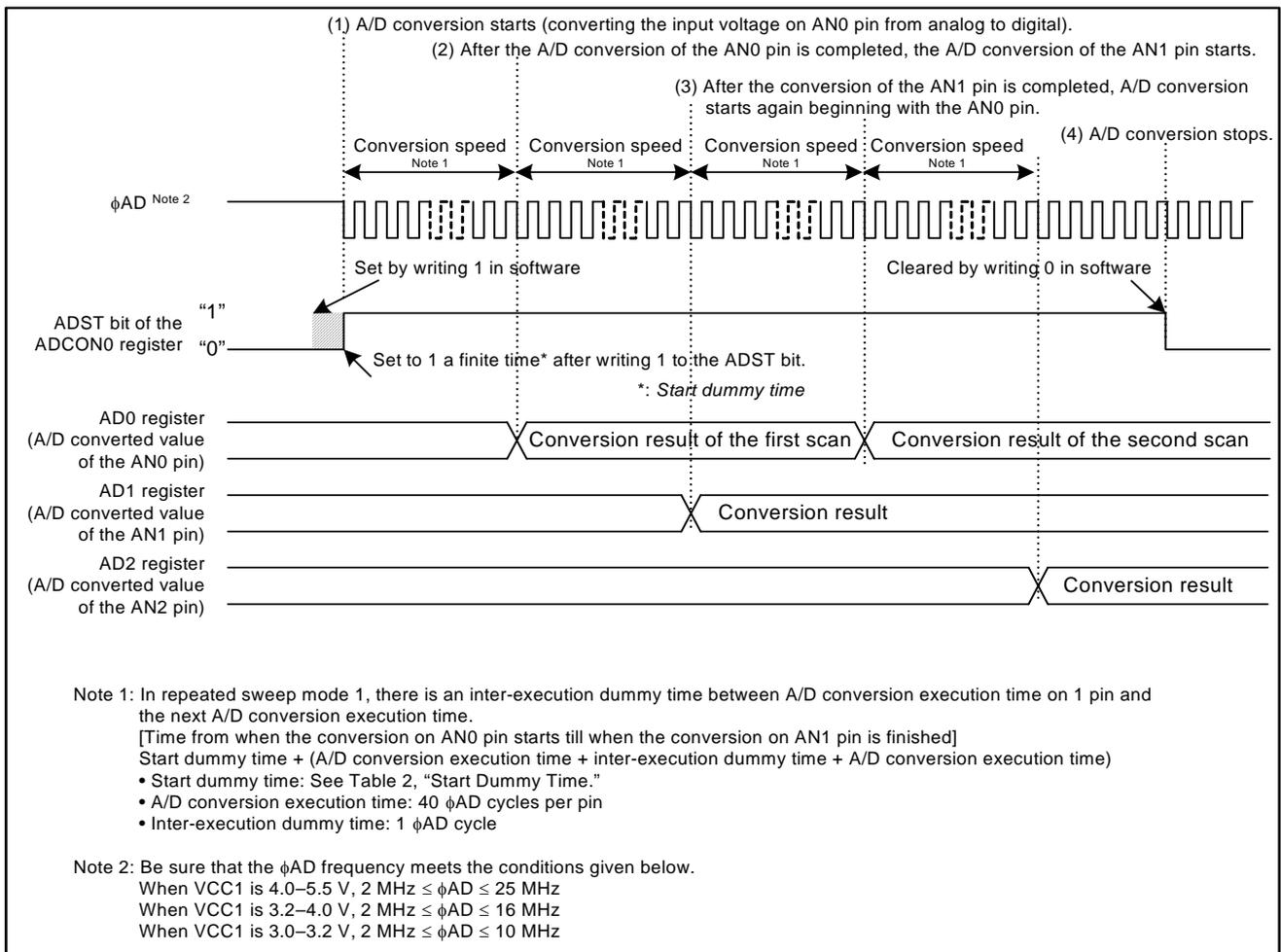
Figure 2. Operation Timing in Repeated Sweep Mode 1
