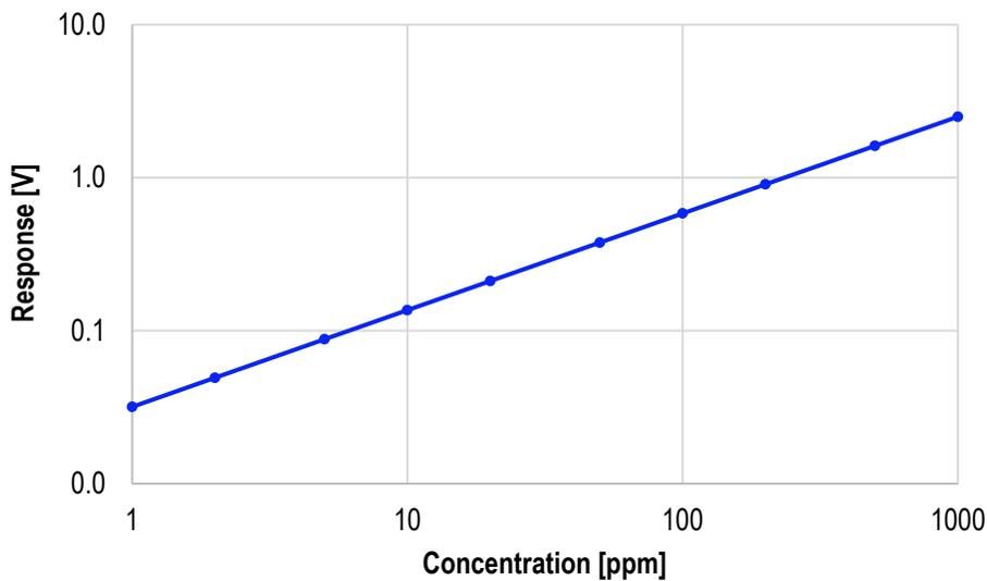
Except for the sensor response change of basis (from (0 to 1) to (0 to 2.5)), the  $\log(response)$  versus  $\log(C)$  plot remains the same.
