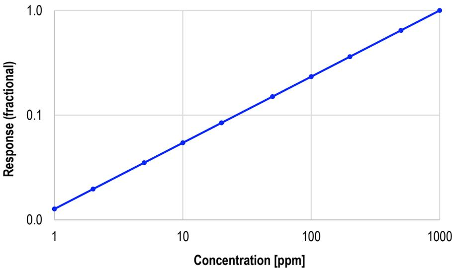
When comparing this plot to the corresponding plot for the voltage divider (Figure 5), it can be seen that there is more responsiveness over the three orders of concentration magnitude in the constant voltage case.
