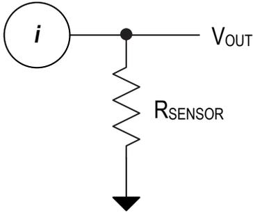
The sensor signal ( $V_{OUT}$ ) relates to sensor resistance according to Equation 14:
