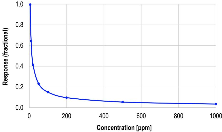
Note that the output signal decreases as gas concentration increases with this type of analog front-end. Also note that linearization of response versus resistance is present in different ways at both low and high gas concentrations, but it is of limited utility because of the “flatness” of the response curve at both ends.
