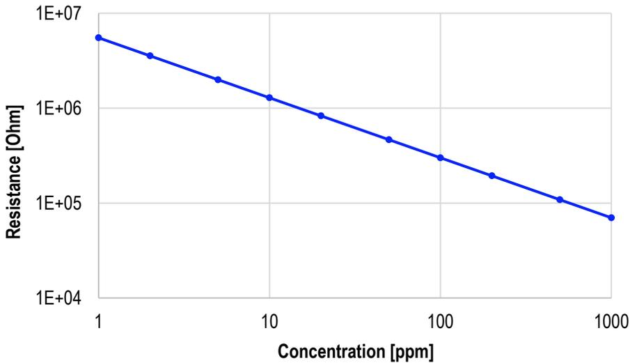
Since simple resistance measurement circuits will have a non-logarithmic transfer function, the fundamental measurement challenge illustrated by Figure 1 is expected when making gas sensor measurements. Additional nonlinear effects from the measurement circuitry exacerbate this challenge and must be understood in order to account for or eliminate these effects.
