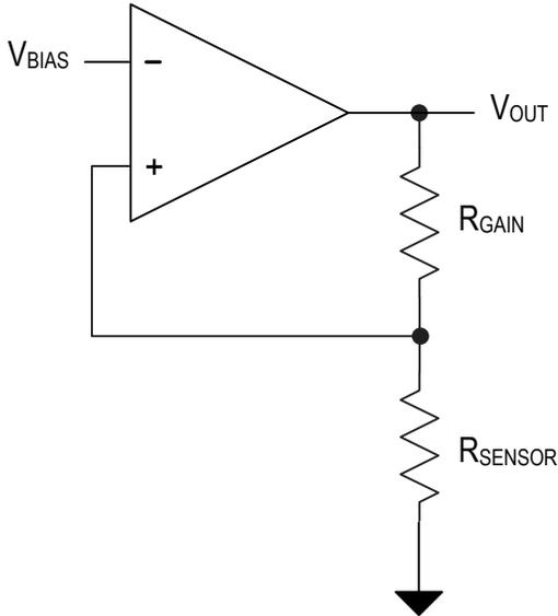
The sensor signal  $V_{OUT}$  relates to sensor resistance according to Equation 9:
