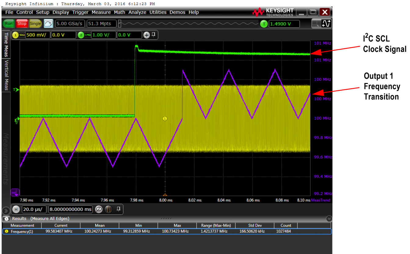
Figure 6. Oscilloscope Image of Output Frequency Transition
