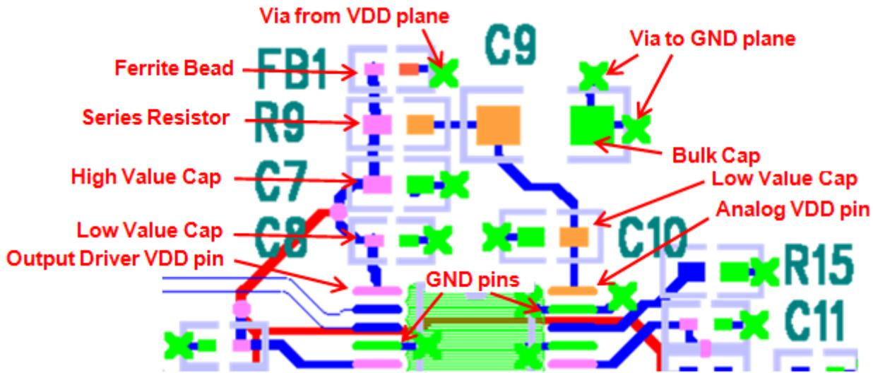
The capacitors most effective at preventing EMI in this layout example are C8 and C10.
