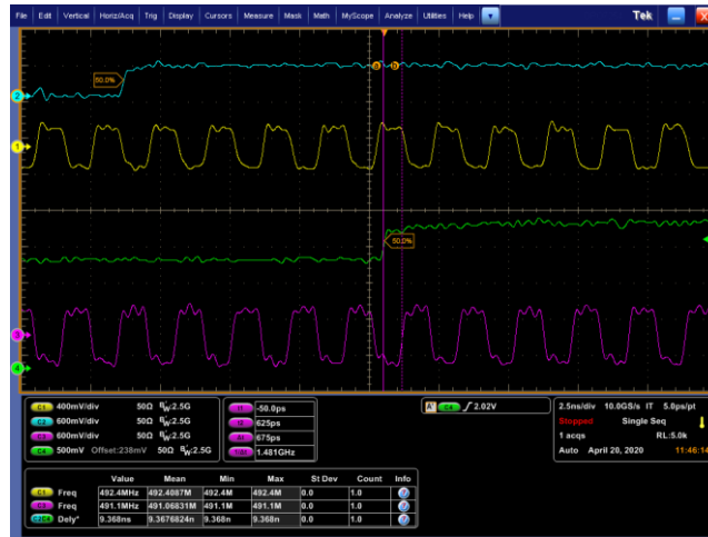
Figure 5. Zoom-In to Show 8V79S680 QREF-to-QCLK Phase Deterministic
