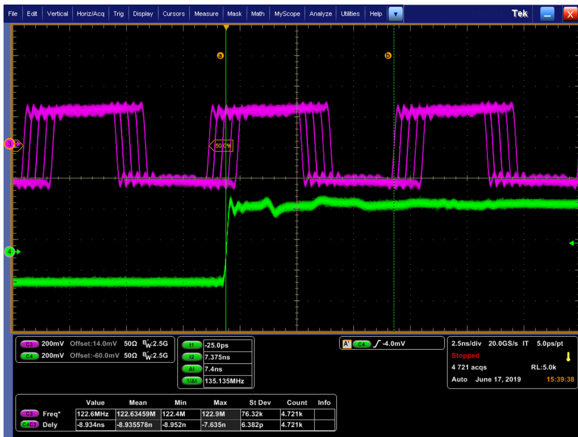
Figure 3. Result of Adjusting Individual Sysref Phase Delay
