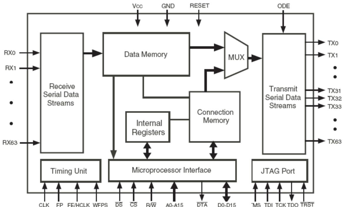
There are two memory blocks shown in [Figure 1](#) - Data Memory and Connection Memory. Data Memory is a temporary buffer of all incoming serial streams. It can be read out by processor to access a particular DS0 in any input serial stream. But its contents can not be altered by system processor.
