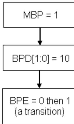
Once a zero-to-one transition is created on BPE bit, the entire Connection Memory block will be initialized in 2 frames (2x125µs = 250µs). The initialization process put A[15:14] = BPD[1:0], A[13:0] = 0x0000 in every single locations in Connection Memory block. By completion, the device will reset BPD[1:0] = 00.
