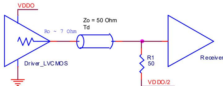
Figure 1. LVCMOS Driver Standard Termination
