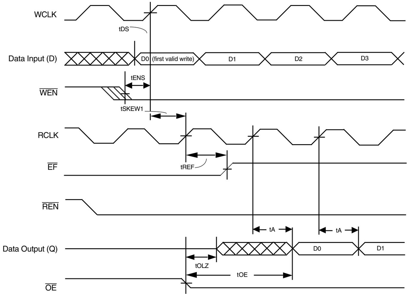
Figure 3. Skew Timing for FIFO#1
