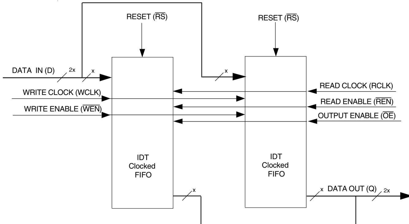
Figure 2. Block Diagram Showing the Control Signals of a SyncFIFO (Clocked FIFO) in a Width Expansion Configuration
