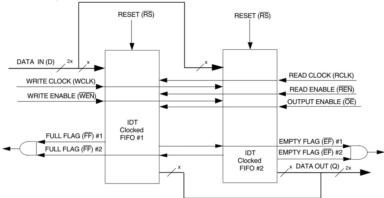
Figure 5. Recommended Block Diagram of Width Expansion using Composite Flags
