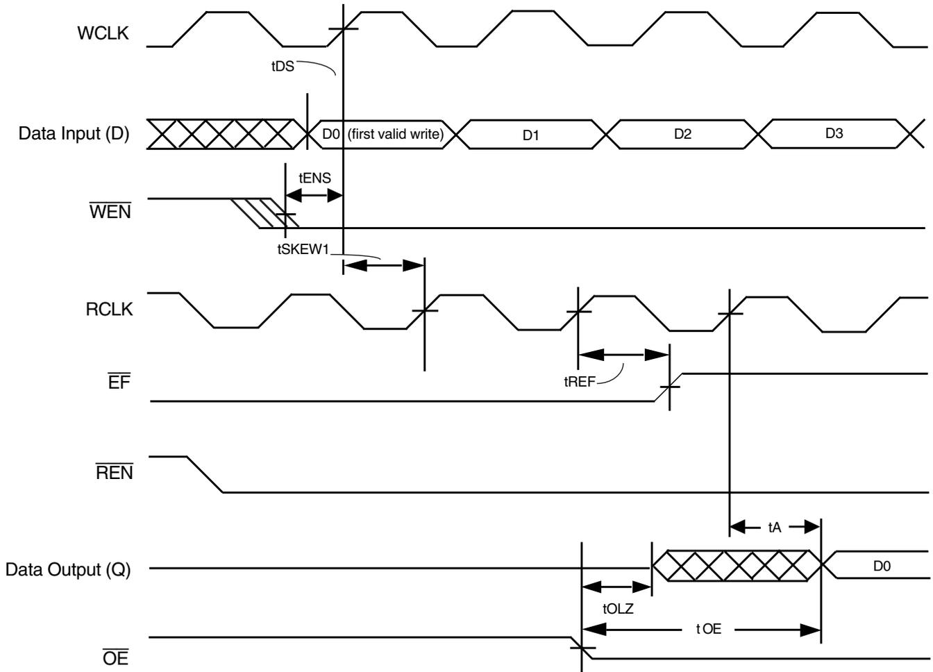
Figure 4. Skew Timing for FIFO#2
