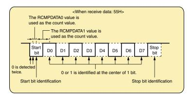
The identification timings are determined by using the <a href="RCMPDATA0">RCMPDATA0</a> value (count value equivalent to 0.5 bits) that was determined via calibration when identifying the start bit, and using the <a href="RCMPDATA1">RCMPDATA1</a> value (count value equivalent to 1 bit) when identifying the bits following bit 0, to identify the timing of the bits at the center of the bits.
