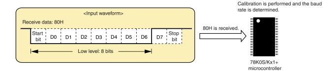
After completion of calibration, 8 units of data are received as a reception test, which are transmitted as a transmission test. Furthermore, an LED is turned on during transmission and reception.
