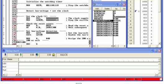
(7) Data transmission and reception will be simulated by software UART and stopped after completion of all processing.
