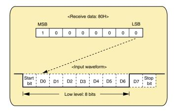
Before starting to measure the low-level width, disable interrupt acknowledgment and set so that no interrupt servicing occurs during the measurement.
