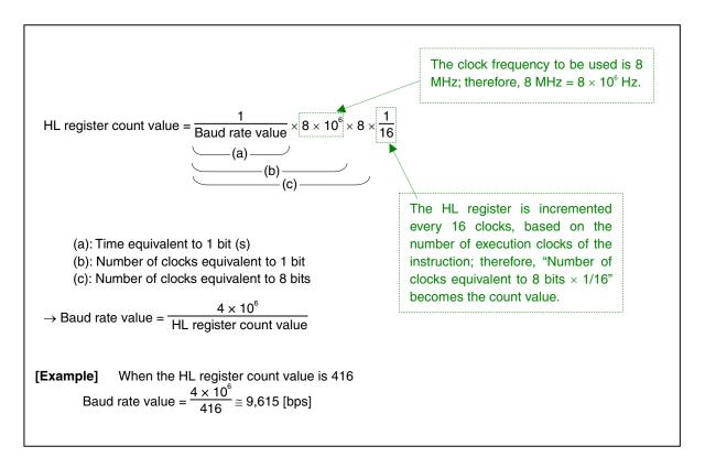
Determine from the value that is a fourth of the HL register count value whether the baud rate is within the recommended range. At this time, the allowable range of the baud rate will be as follows, based on the identified value of the count value.
