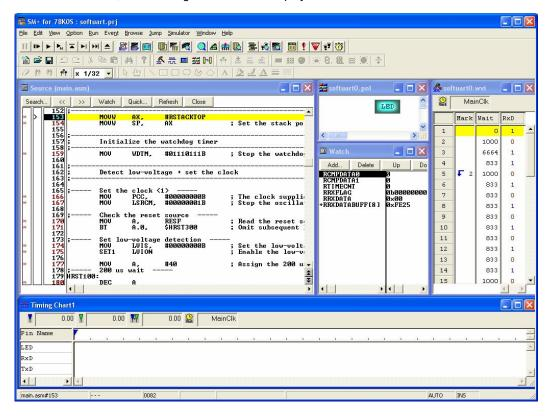
(3) The first character changes from a plus sign ("+") to a minus sign ("-") and the receive data to be saved will be expanded and displayed below "-RRXDATABUFF [8]", by selecting the watch window (Watch) and double-clicking "+RRXDATABUFF [8]".
