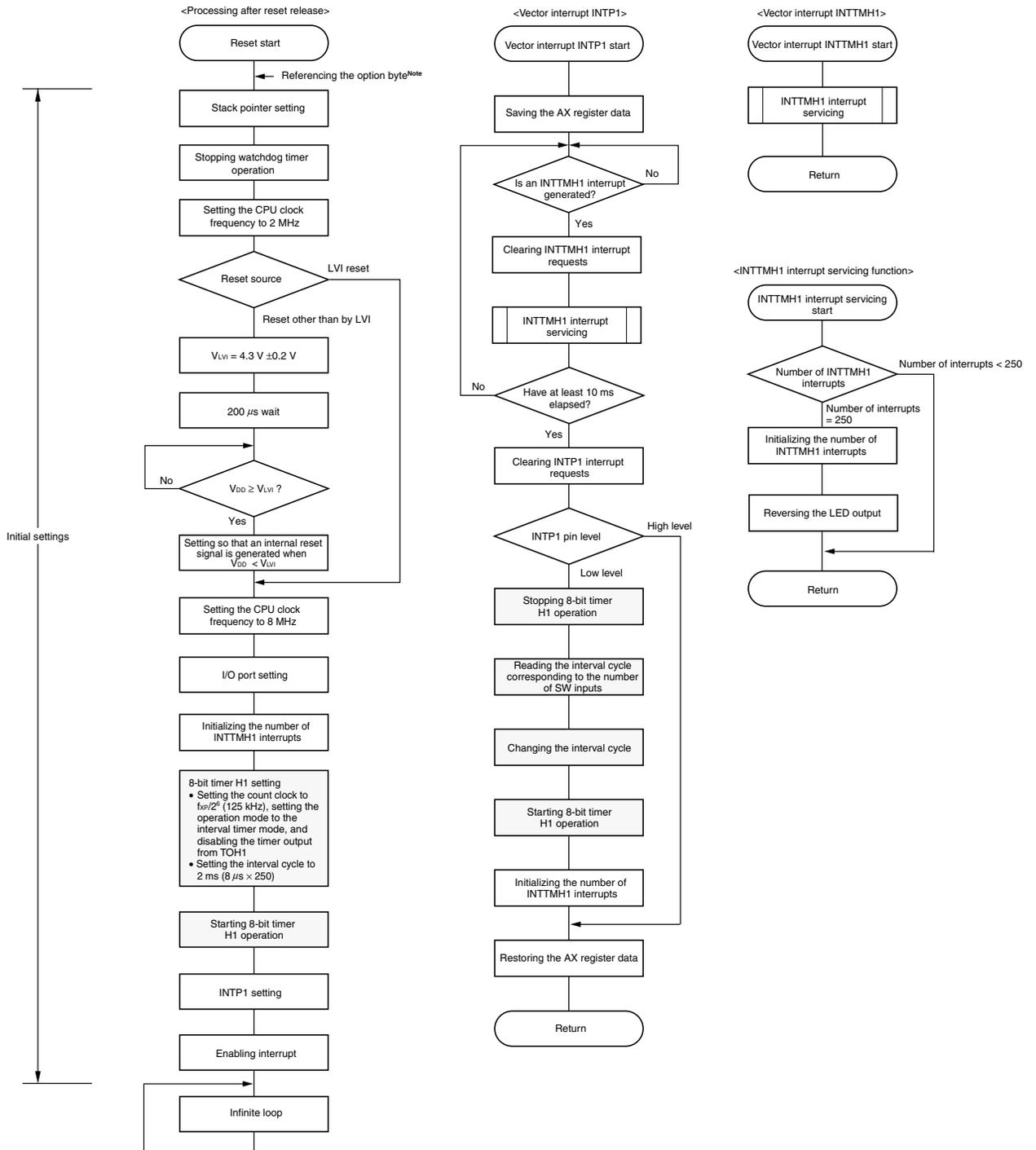
**Note** Referencing the option byte is automatically performed by the microcontroller after reset release. In this sample program, the following contents are set by referencing the option byte.
