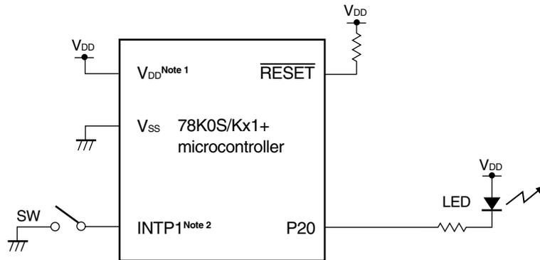
**Notes** 1. Use this in a voltage range of  $4.5\text{ V} \leq V_{DD} \leq 5.5\text{ V}$ .
