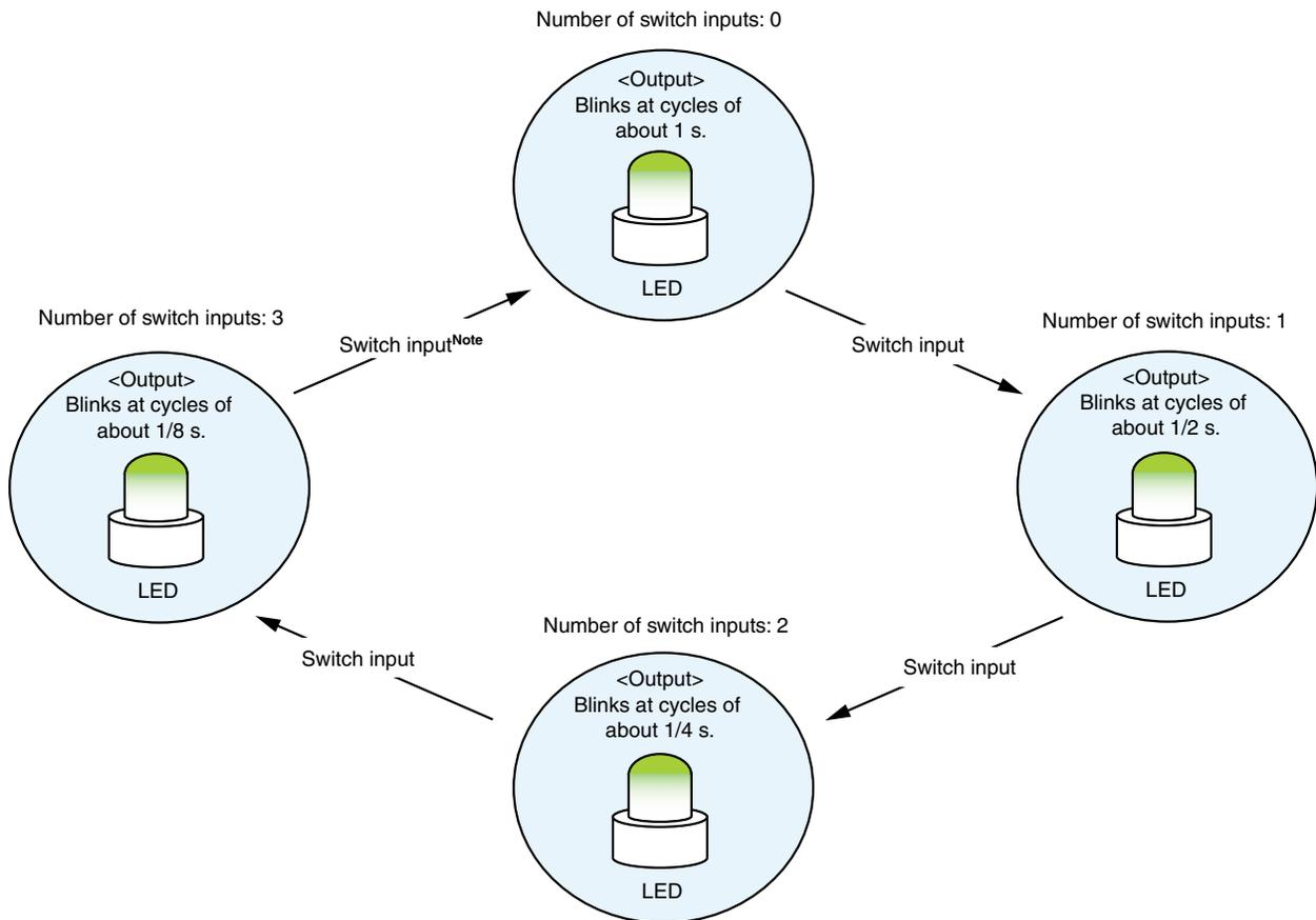
**Note** The blinking cycle from the zeroth switch input is repeated after the fourth switch input.
