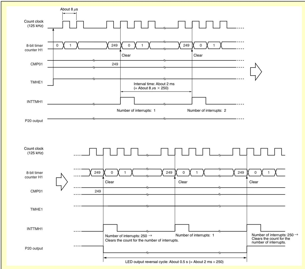
**Remark** The CMP01 register setting value is 124, 62, and 31 when the LEDs blink at respective cycles of about 1/2 s, 1/4 s, and 1/8 s.
