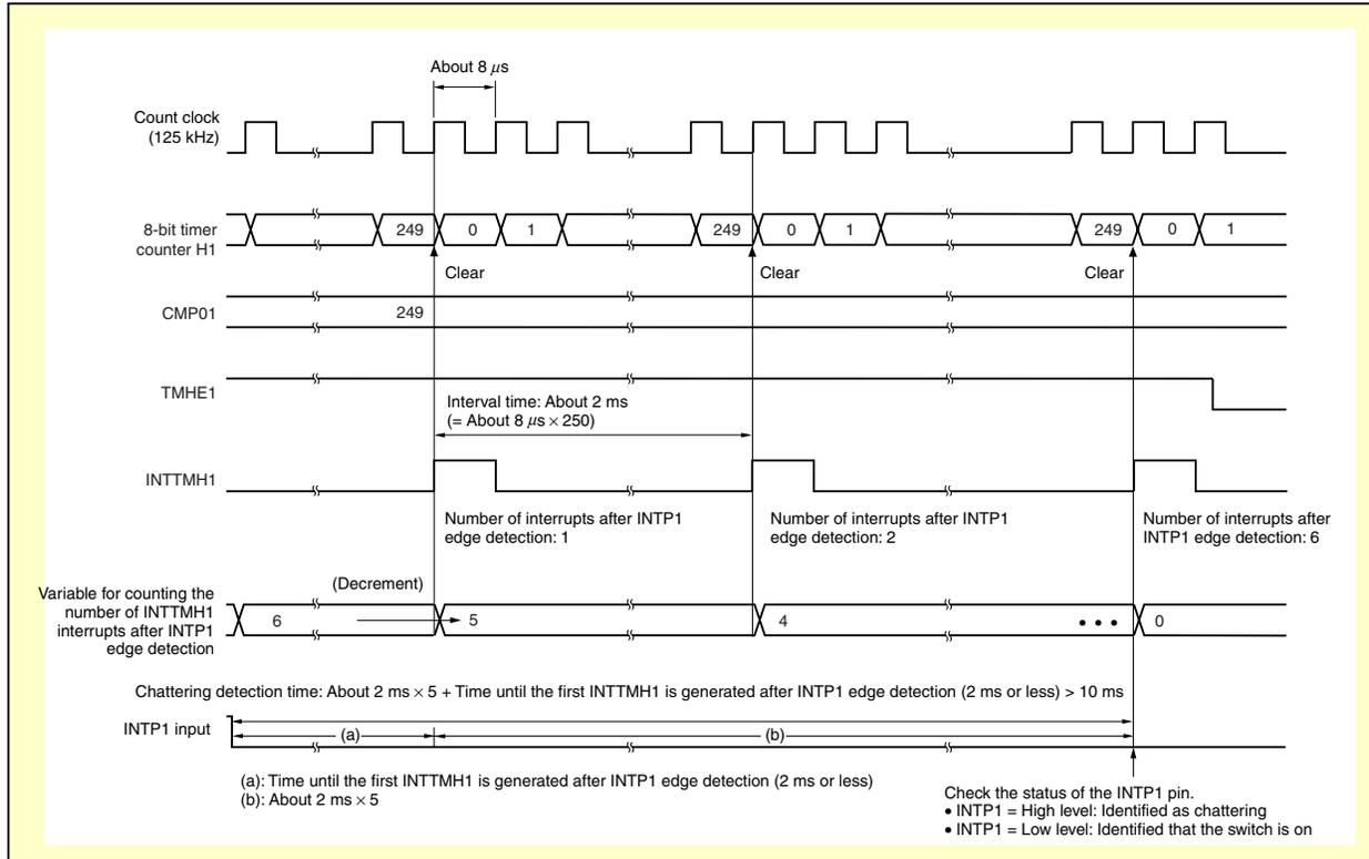
**Remark** The variable for counting the number of INTTMH1 interrupts after INTP1 edge detection depends on the LED blinking cycle during switch input. The variable is 11, 21, and 41, when the LEDs blink at respective cycles of about 1/2 s, 1/4 s, and 1/8 s.
