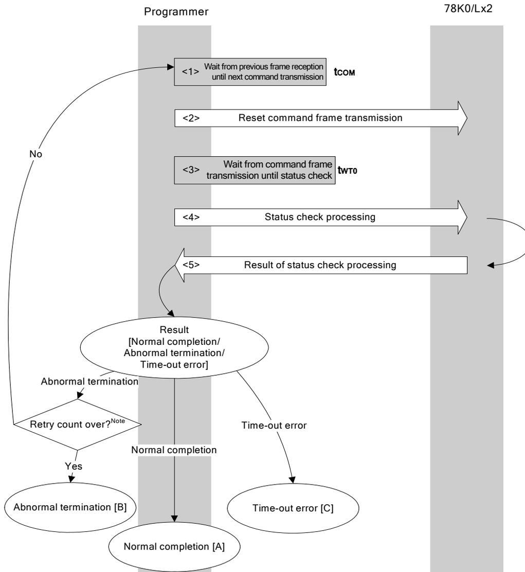
**Note** Do not exceed the retry count for the reset command transmission (up to 16 times).
