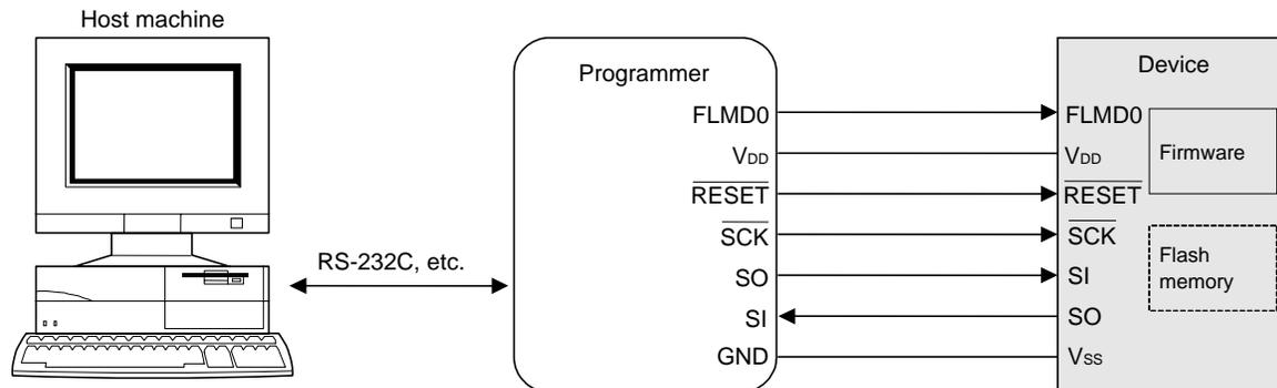
**Remark** As for the pins used for flash memory programming and the recommended connections of unused pins, see the user's manual of each product.
