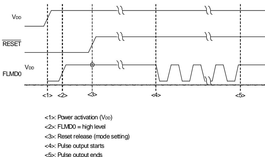
The relationship between the setting of the FLMD0 pin after reset release and the operating mode is shown below.
