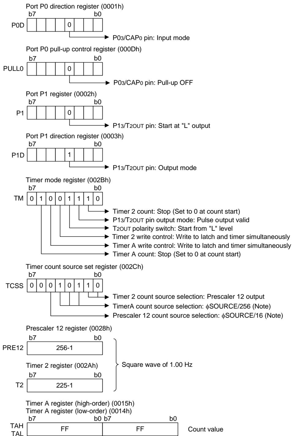
Note:  $\phi$ SOURCE is the clock selected by bits 5 and 4 at the clock mode register (address 0037h). Timer count sources are not affected by bits 7 and 6 (clock dividing ratio selection bits).
