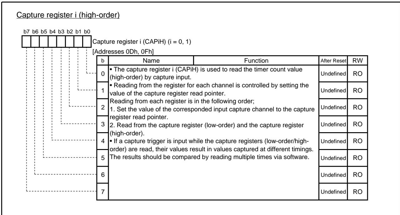
Fig.4.12 Configuration of Capture register i (high-order)
