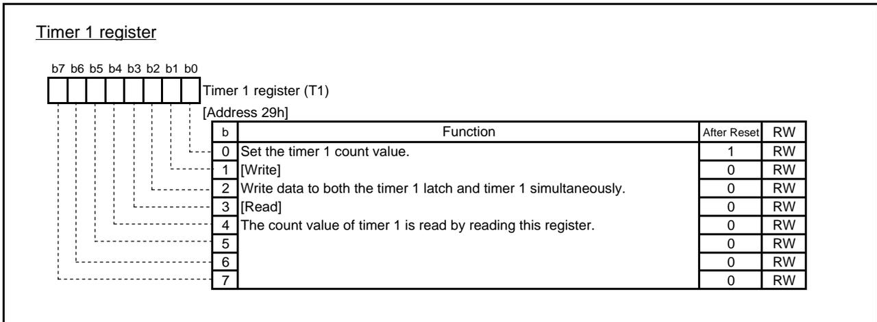
Fig.4.36 Configuration of Timer 1 register
