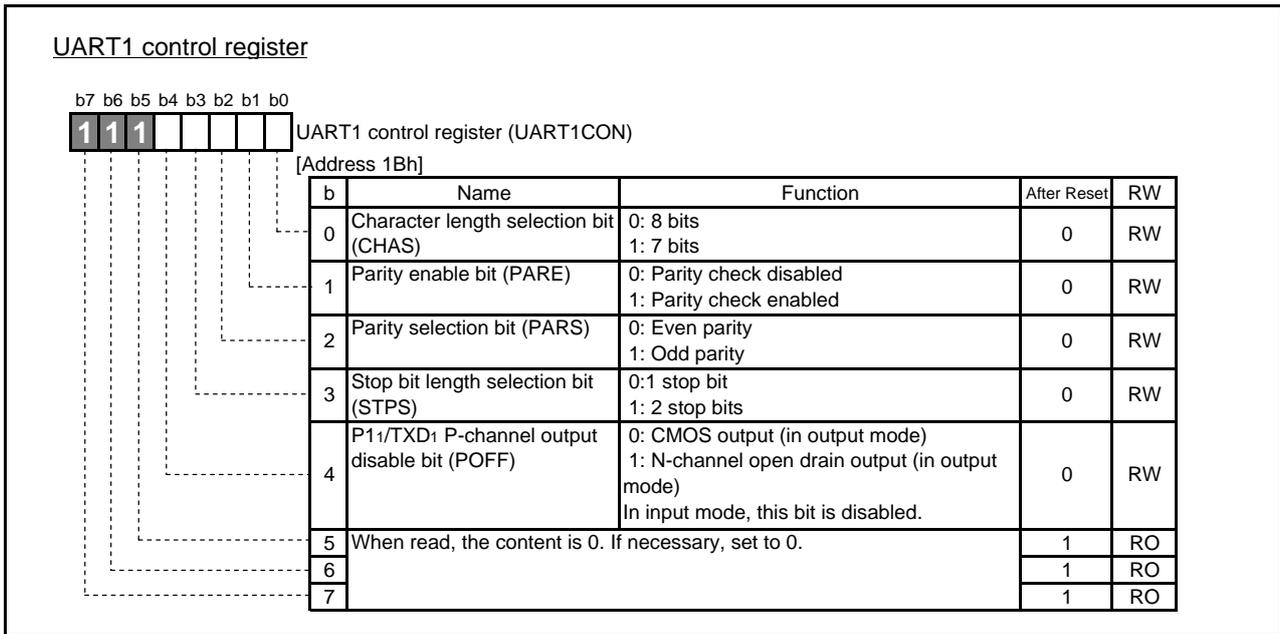
Fig. 4.24 Configuration of UART1 control register
