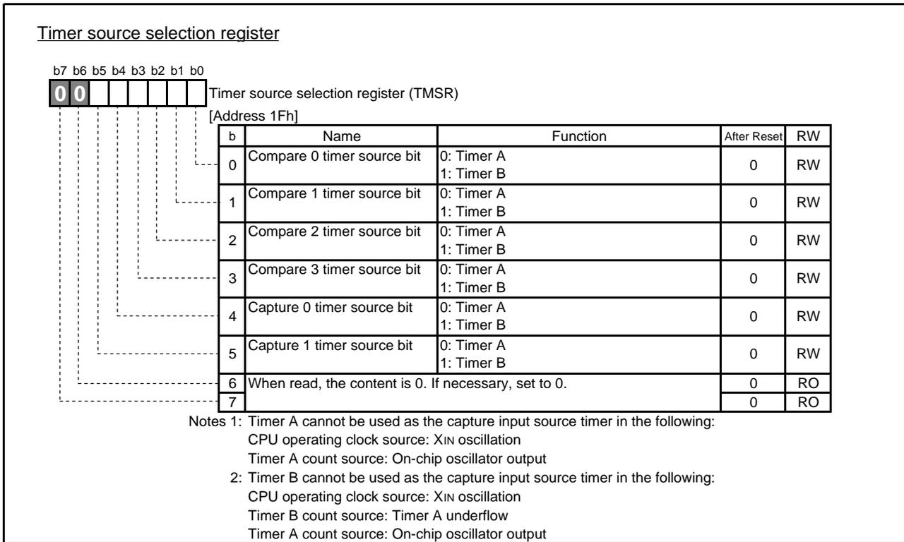
Fig.4.28 Configuration of Timer source selection register
