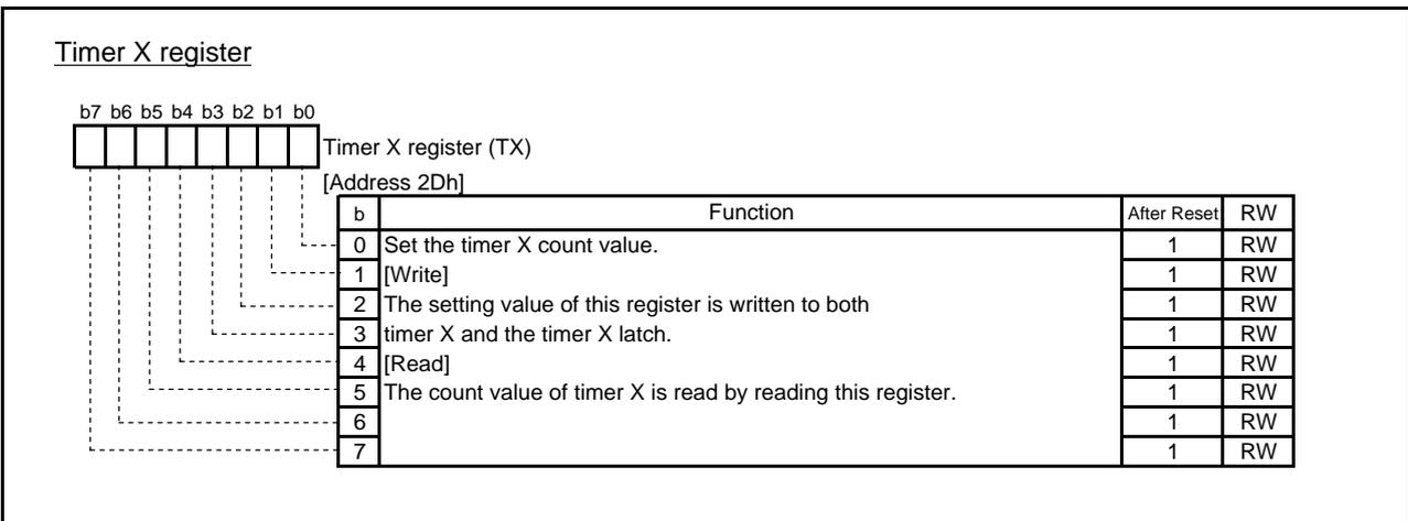
Fig.4.40 Configuration of Timer X register
