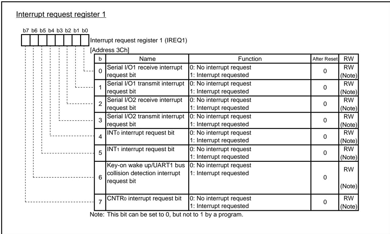
Fig.4.54 Configuration of Interrupt request register 1
