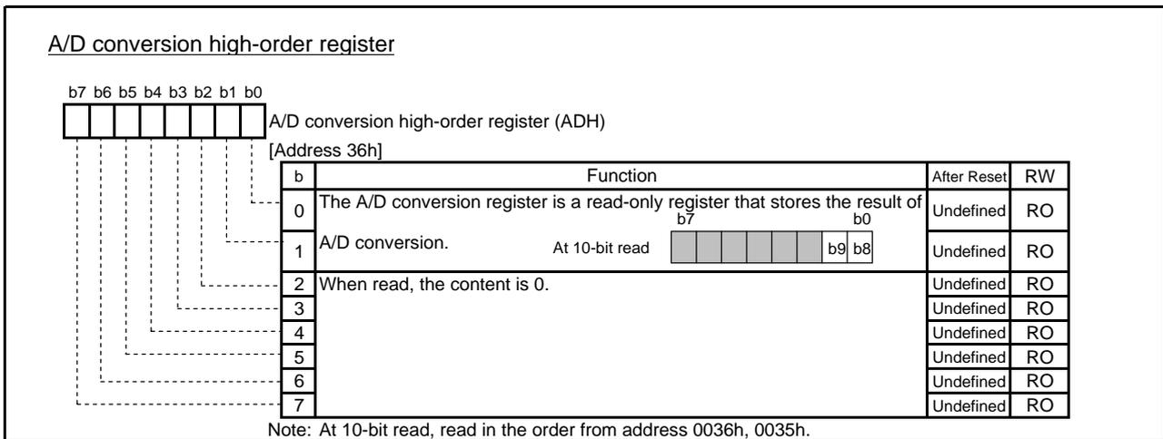
Fig.4.48 Configuration of A/D conversion high-order register
