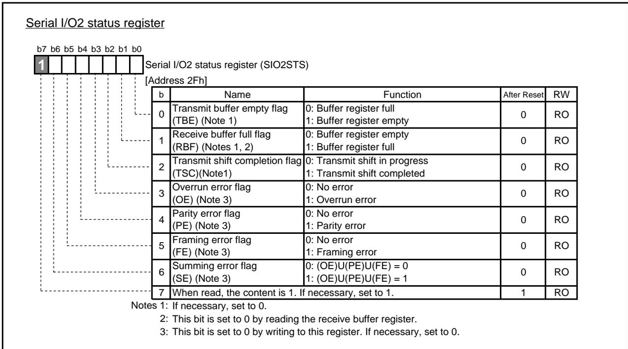
Fig.4.42 Configuration of Serial I/O2 status register
