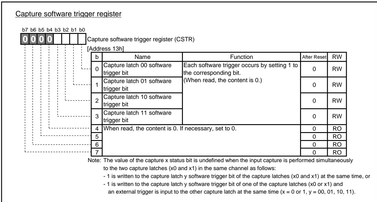
Fig. 4.16 Configuration of Capture software trigger register
