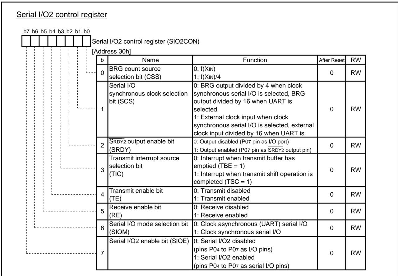
Fig.4.43 Configuration of Serial I/O2 control register
