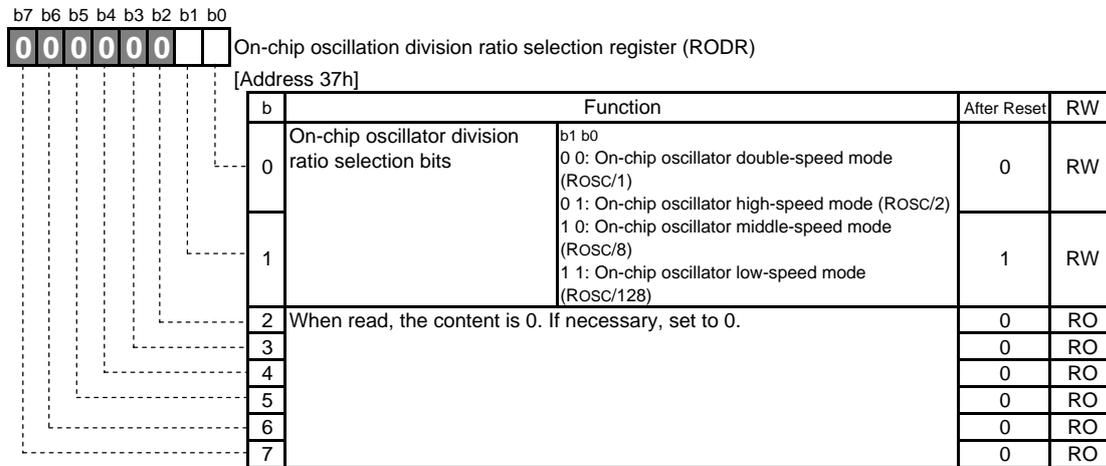
Fig.4.49 Configuration of On-chip oscillation division ratio selection register
