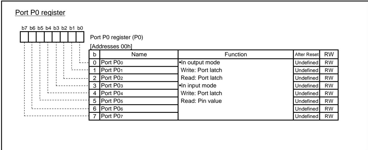
Fig. 4.1 Configuration of Port P0 register
