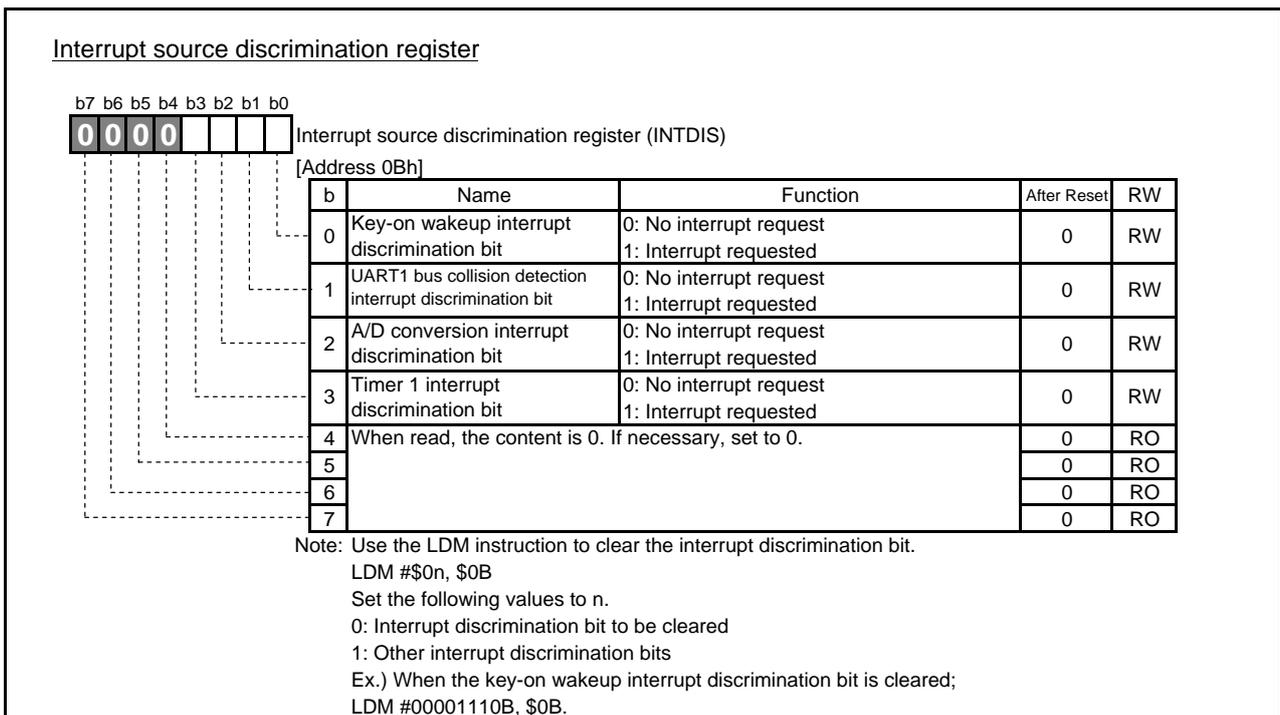
Fig. 4.10 Configuration of Interrupt source discrimination register
