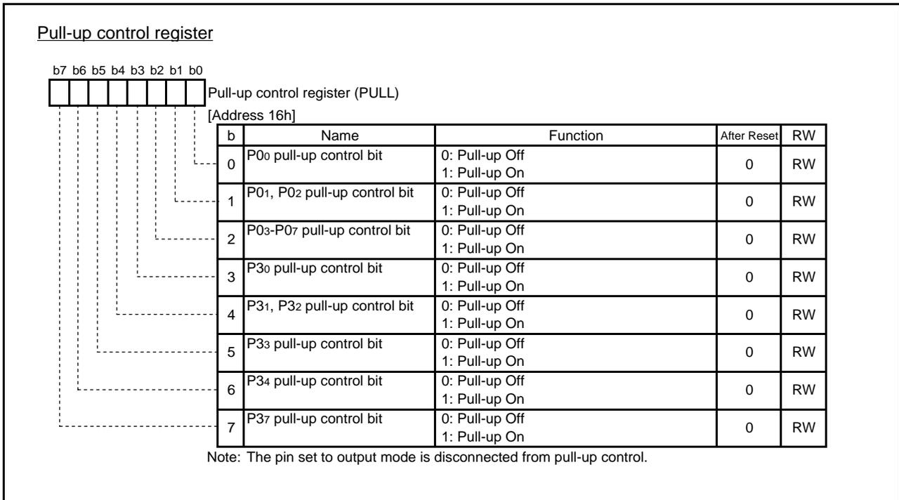
Fig. 4.19 Configuration of Pull-up control register
