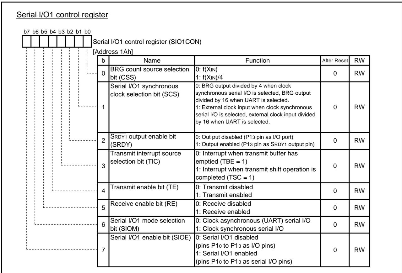
Fig. 4.23 Configuration of Serial I/O1 control register
