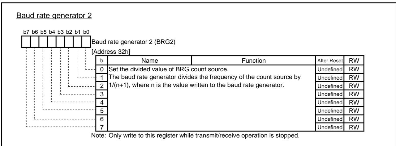
Fig.4.45 Configuration of Baud rate generator 2
