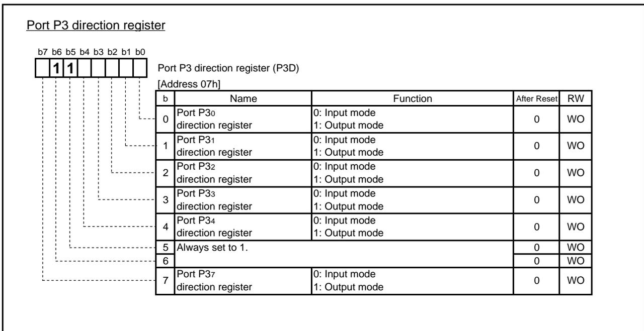
Fig. 4.8 Configuration of Port P3 direction register
