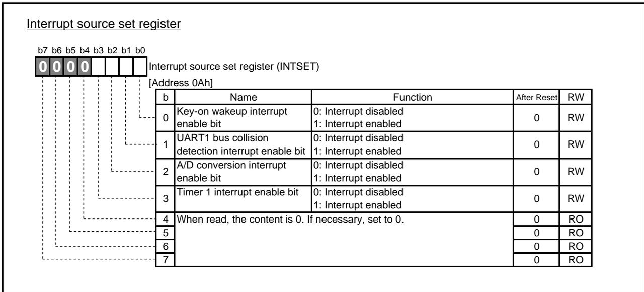
Fig. 4.9 Configuration of Interrupt source set register
