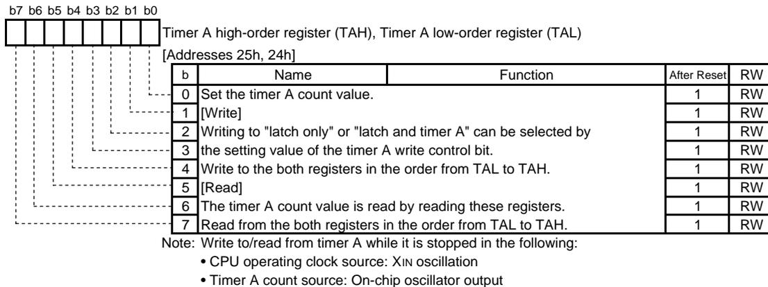
Fig.4.33 Configuration of Timer A high-order register, Timer A low-order register
