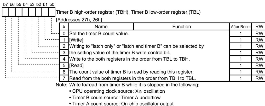
Fig.4.34 Configuration of Timer B high-order register, Timer B low-order register
