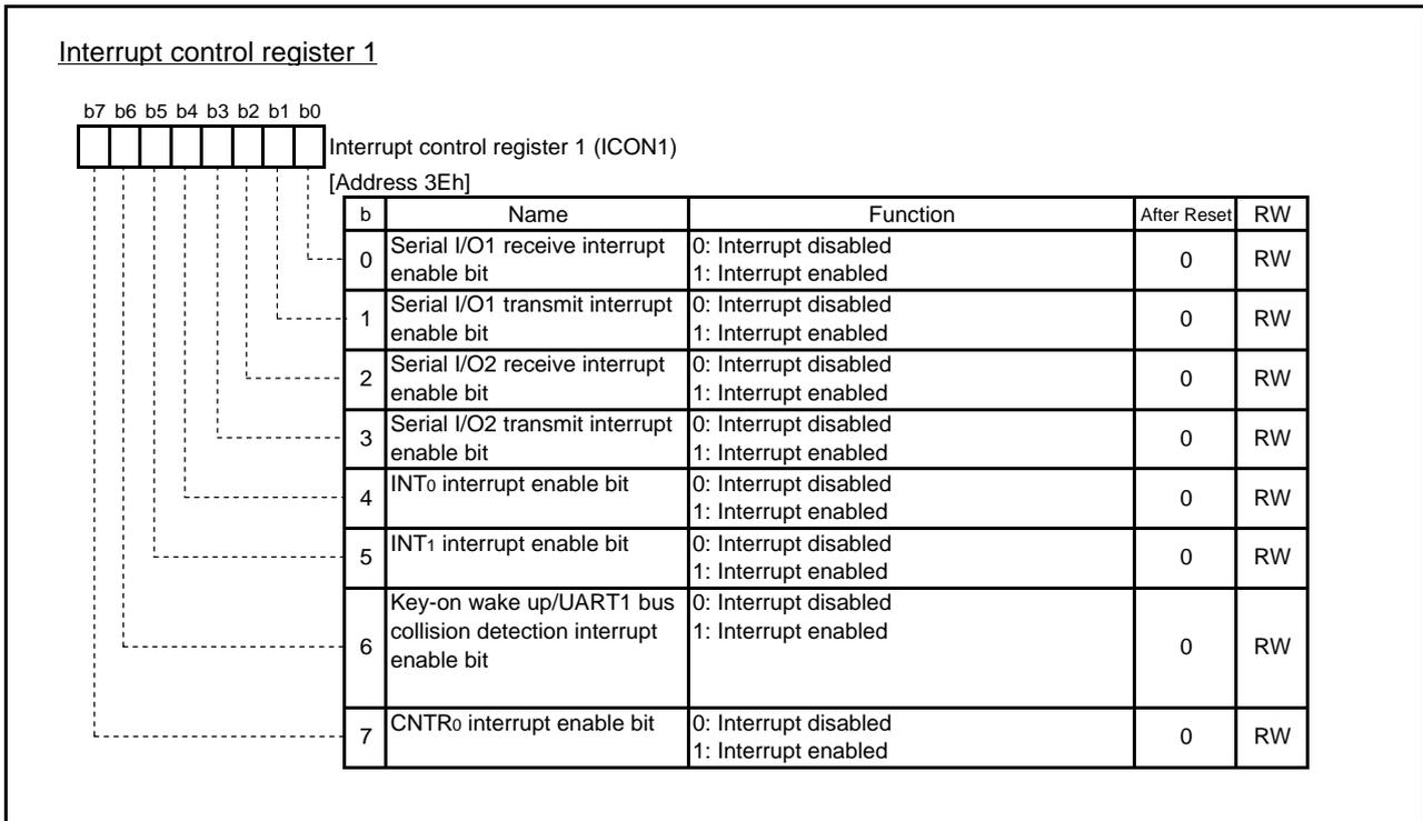
Fig.4.56 Configuration of Interrupt control register 1
