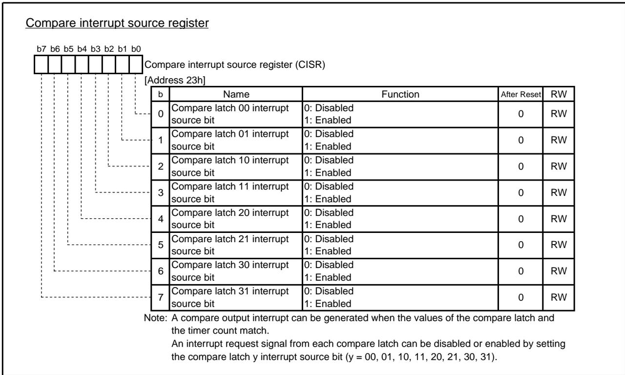
Fig.4.32 Configuration of Compare interrupt source register
