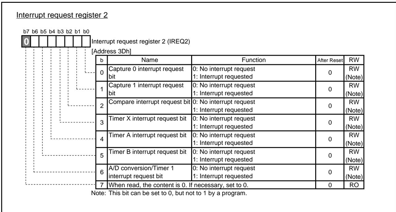
Fig.4.55 Configuration of Interrupt request register 2
