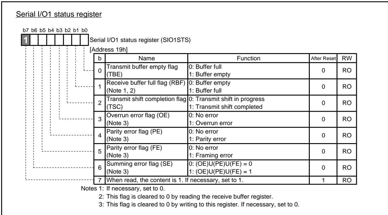
Fig. 4.22 Configuration of Serial I/O1 status register
