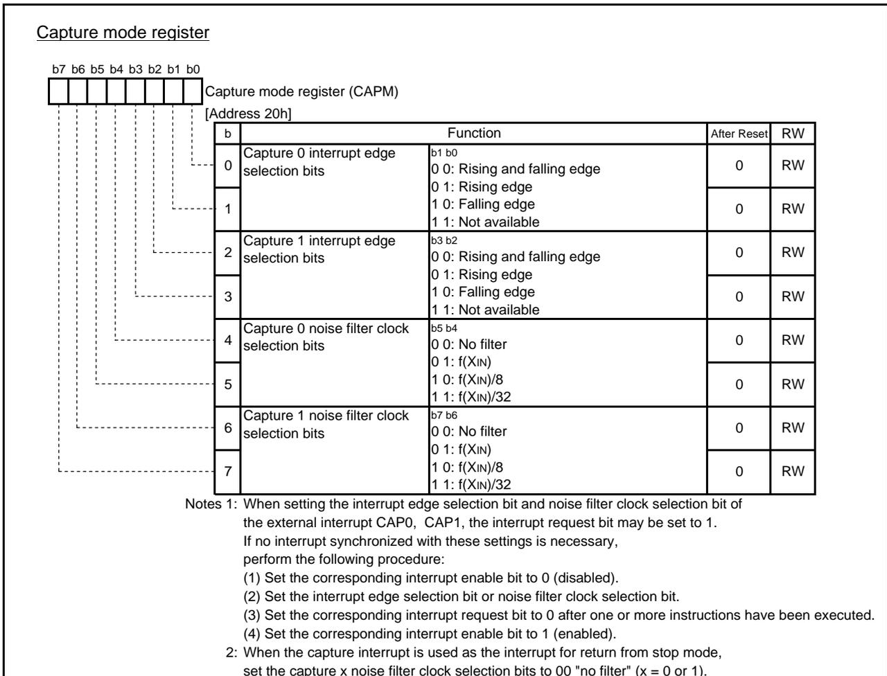
Fig.4.29 Configuration of Capture mode register
