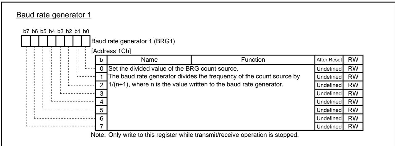
Fig.4.25 Configuration of Baud rate generator 1
