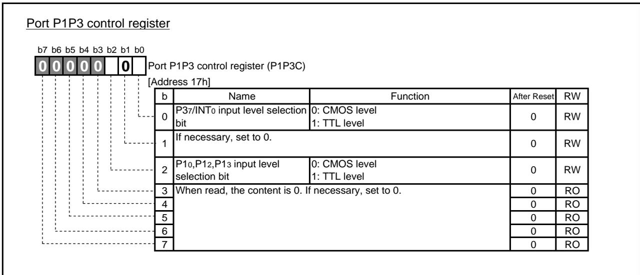
Fig. 4.20 Configuration of Port P1P3 control register
