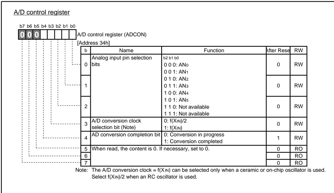
Fig.4.46 Configuration of A/D control register
