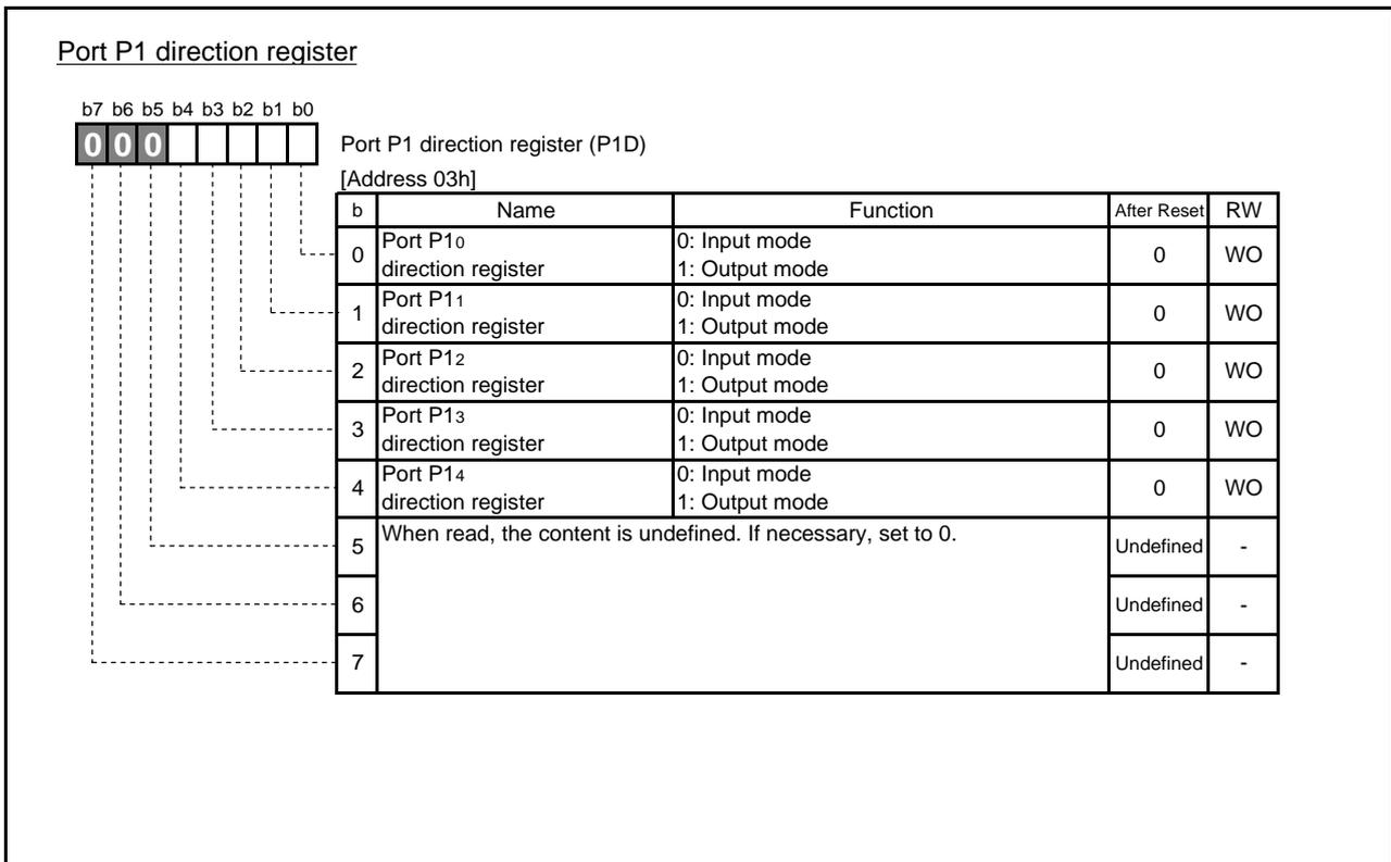
Fig. 4.4 Configuration of Port P1 direction register
