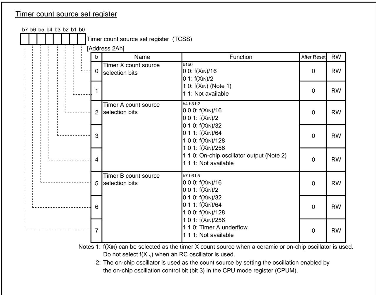
Fig.4.37 Configuration of Timer count source set register
