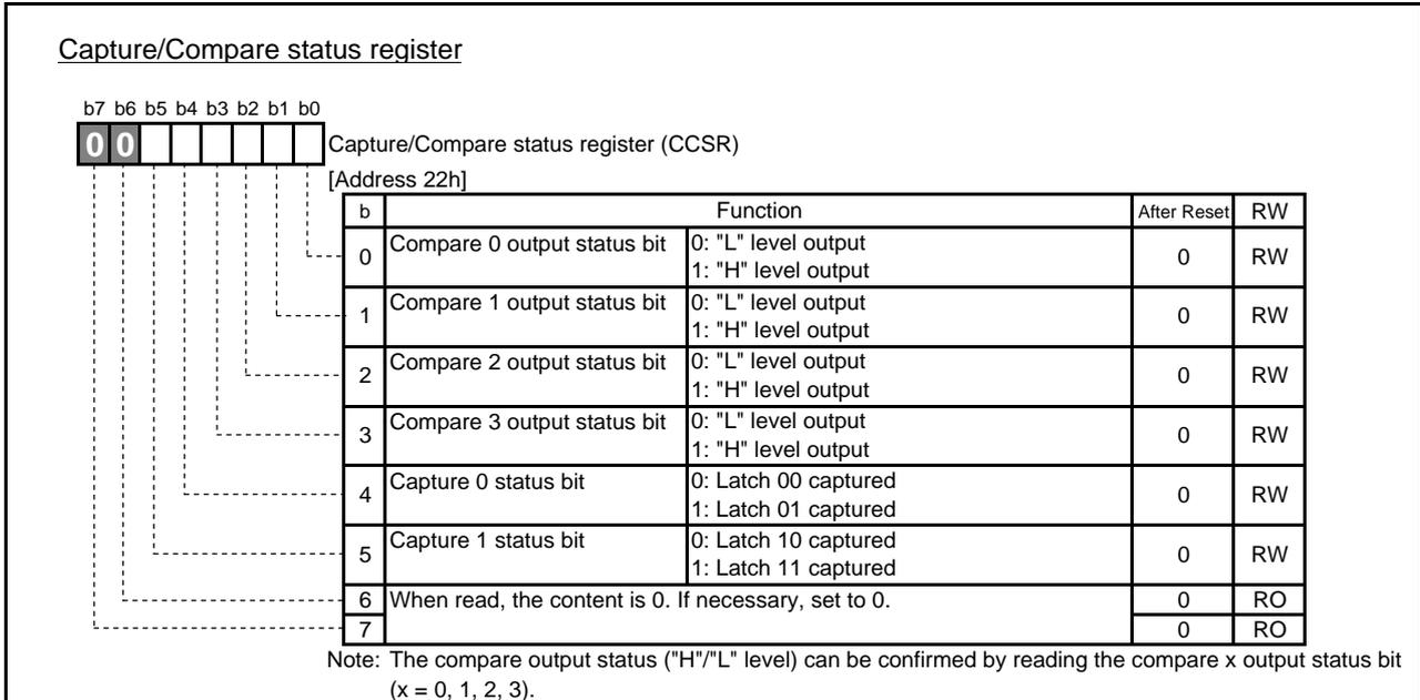
Fig.4.31 Configuration of Capture/Compare status register
