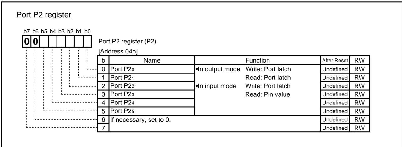
Fig. 4.5 Configuration of Port P2 register
