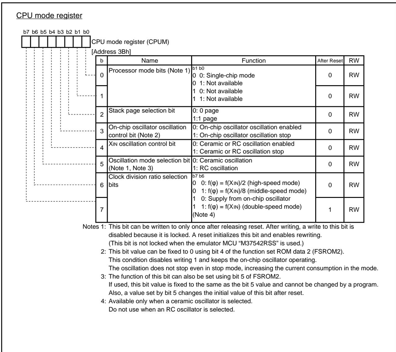
Fig.4.53 Configuration of CPU mode register
