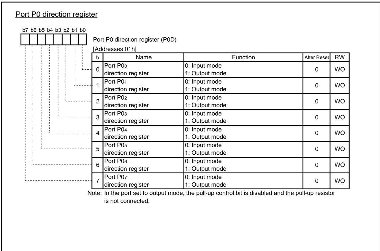
Fig. 4.2 Configuration of Port P0 direction register
