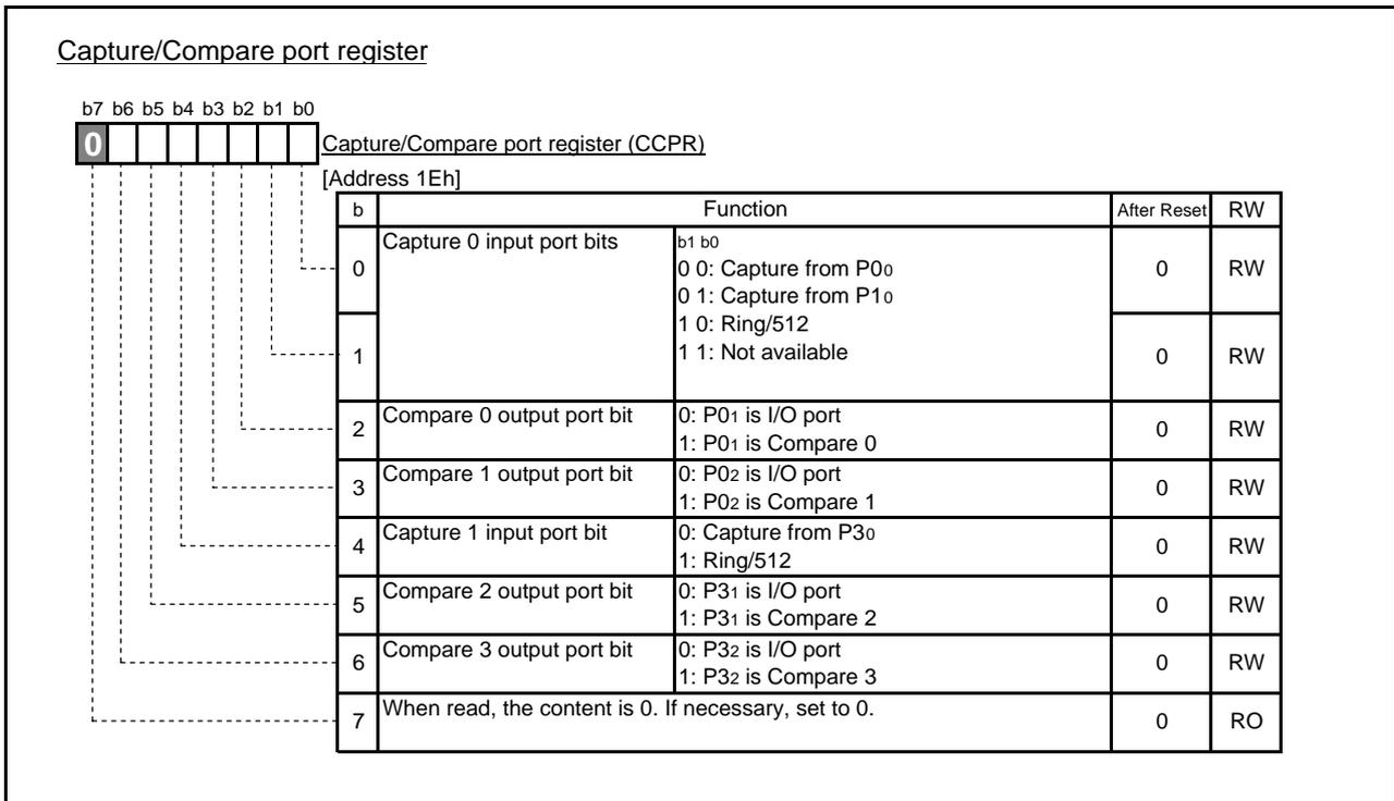
Fig.4.27 Configuration of Capture/Compare port register
