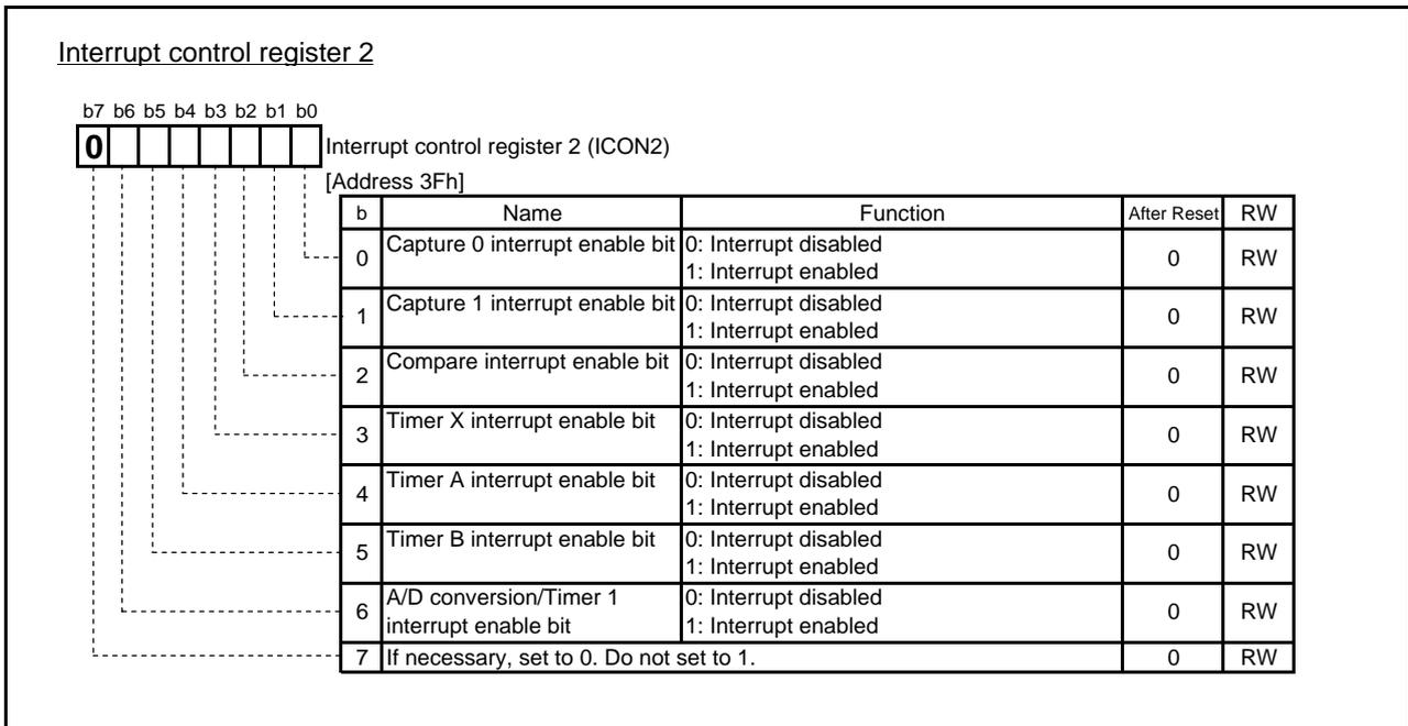
Fig.4.57 Configuration of Interrupt control register 2
