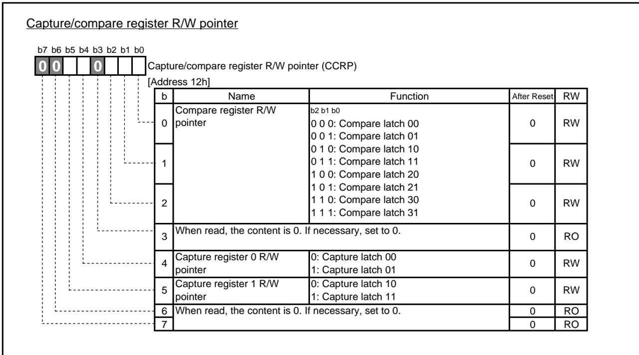
Fig. 4.15 Configuration of Capture/compare register R/W pointer
