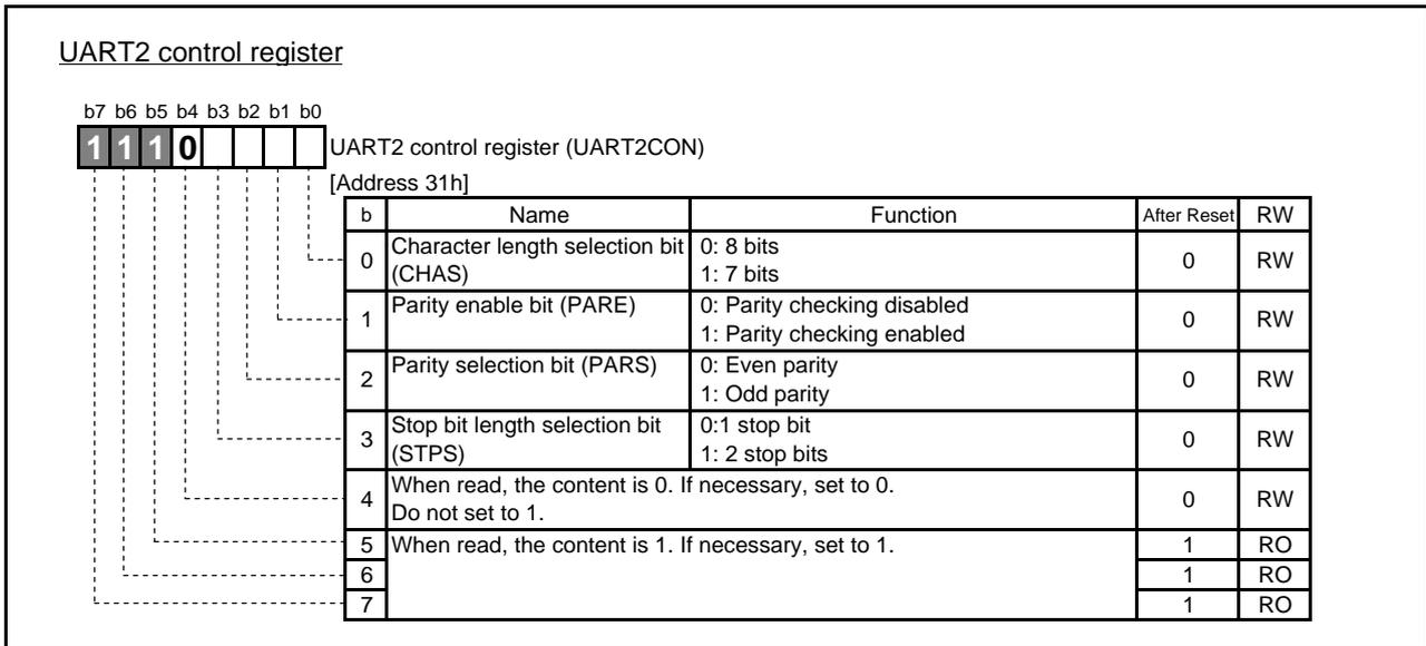
Fig.4.44 Configuration of UART2 control register
