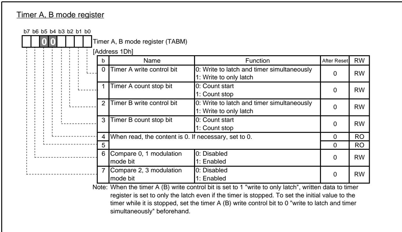
Fig.4.26 Configuration of Timer A, B mode register
