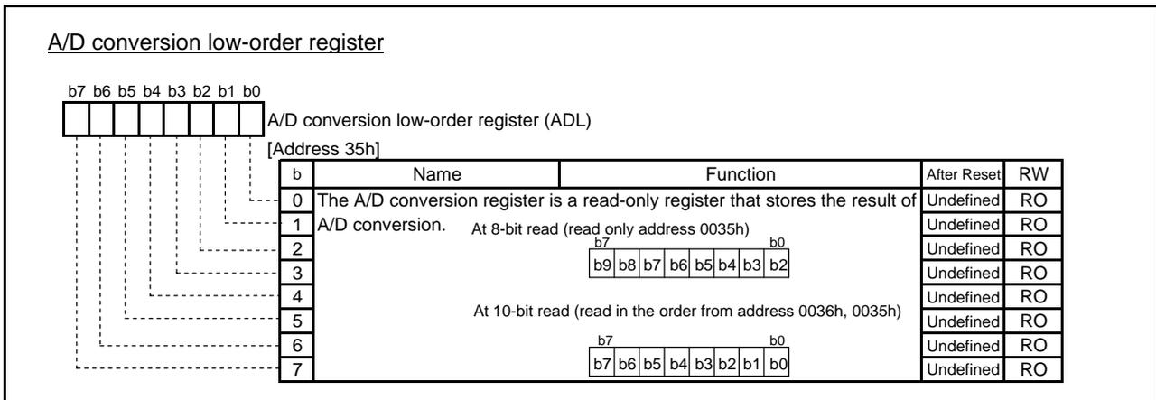
Fig.4.47 Configuration of A/D conversion low-order register
