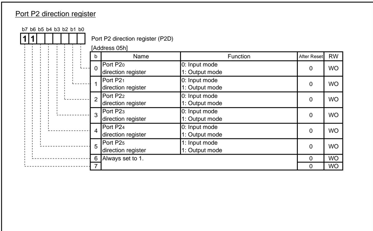
Fig. 4.6 Configuration of Port P2 direction register
