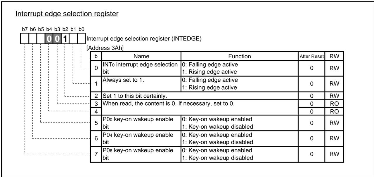
Fig.4.52 Configuration of Interrupt edge selection register
