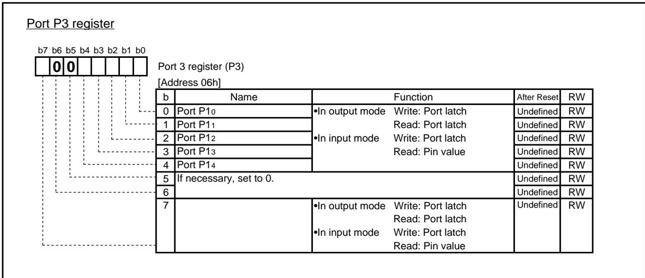
Fig. 4.7 Configuration of Port P3 register
