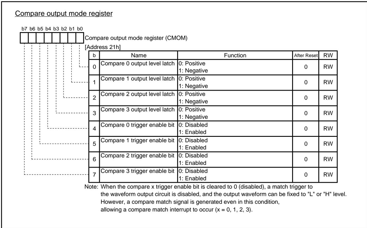
Fig.4.30 Configuration of Compare output mode register
