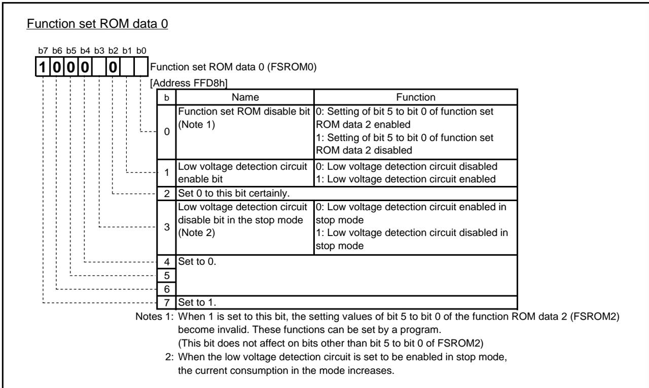
Fig.4.58 Configuration of Function set ROM data 0
