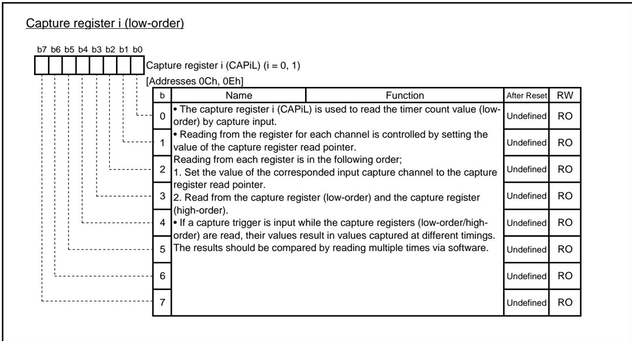
Fig.4.11 Configuration of Capture register i (low-order)
