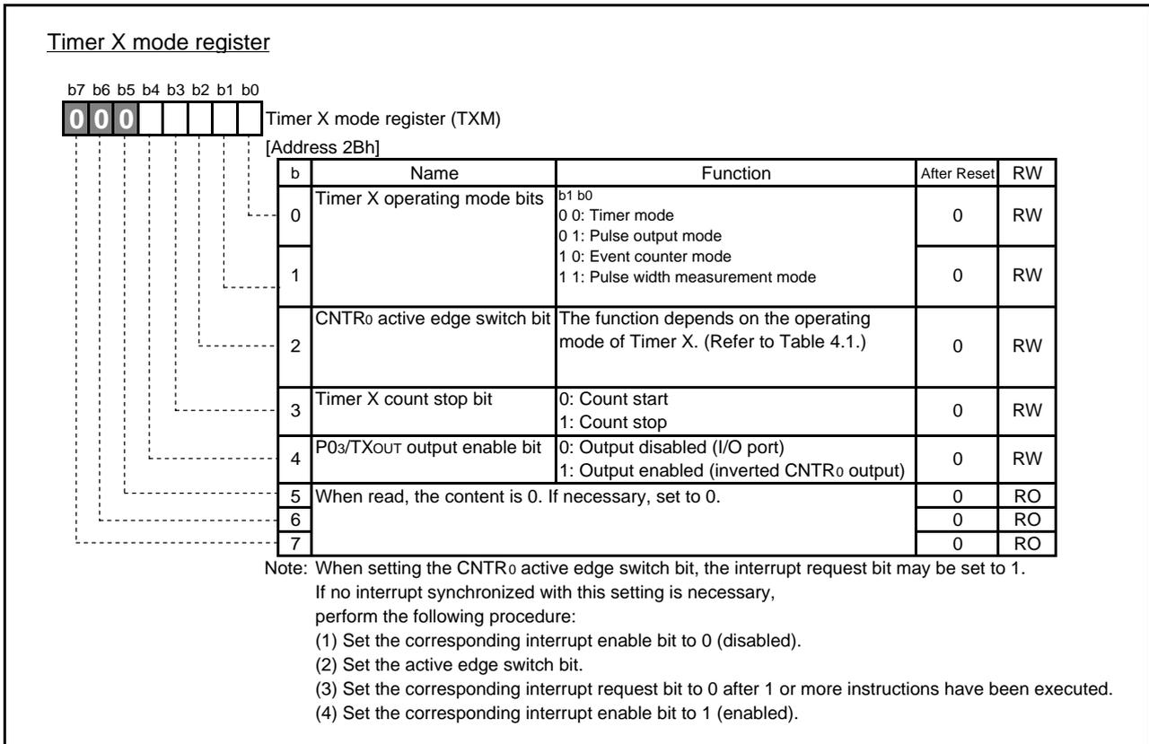
Fig.4.38 Configuration of Timer X mode register
