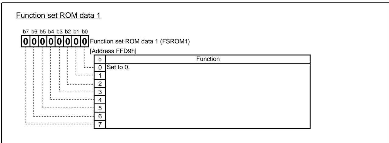
Fig.4.59 Configuration of Function set ROM data 1
