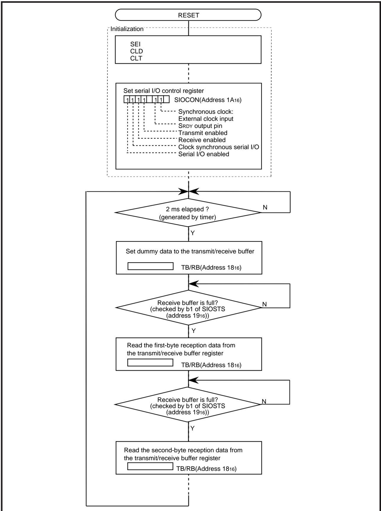
Figure 6 Control procedure of receiver
