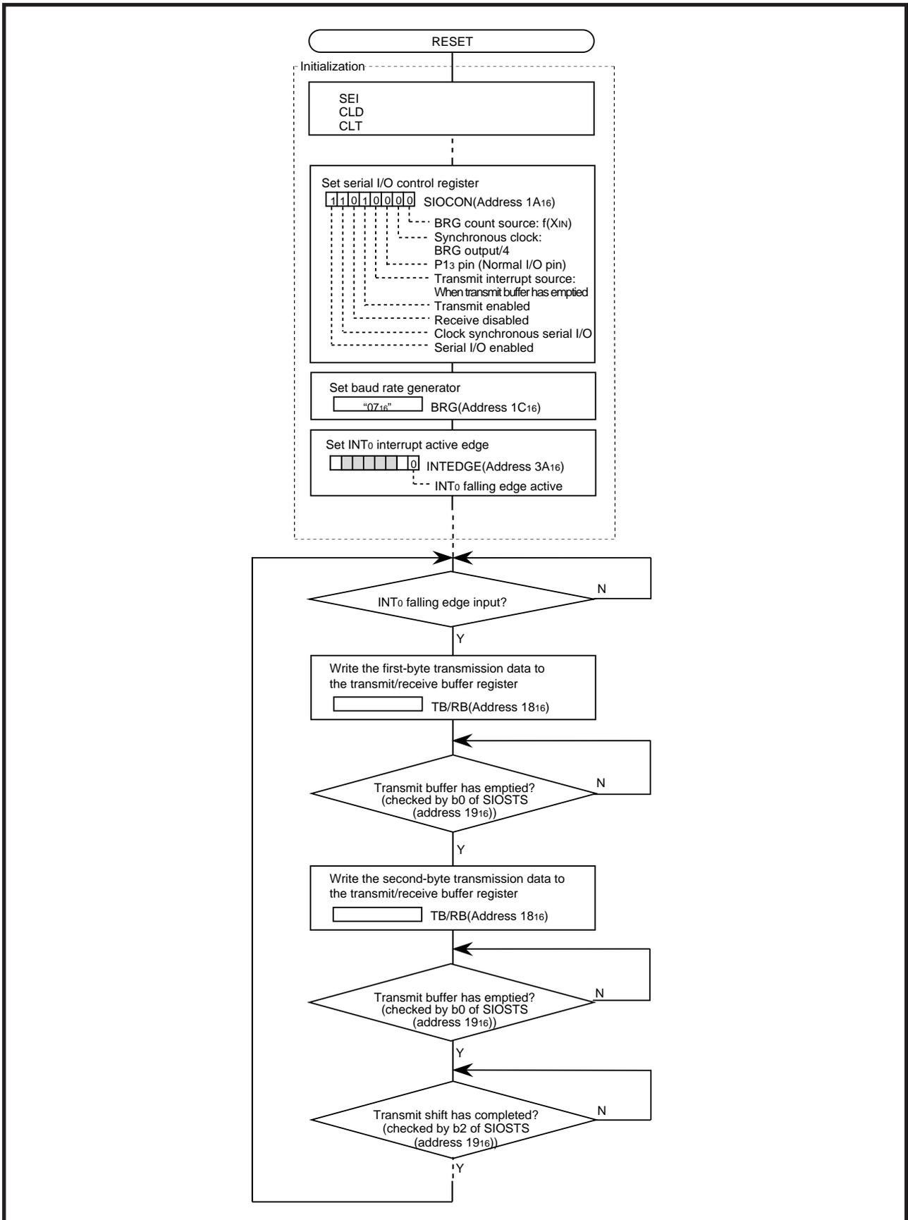
Figure 5 Control procedure of transmitter
