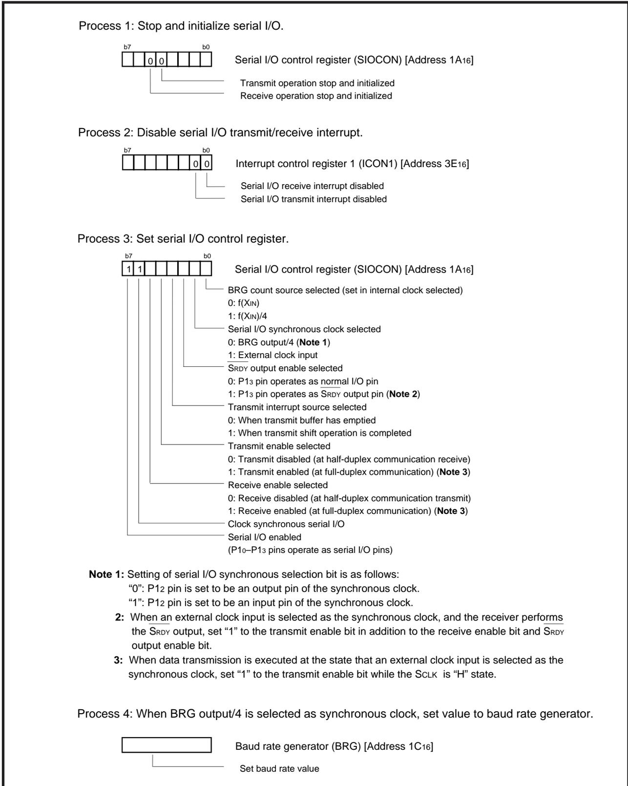
Figure 1 Setting method for clock synchronous serial I/O (1)
