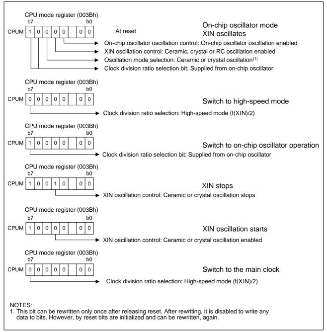
Figure 3.2 Relevant Register Settings
