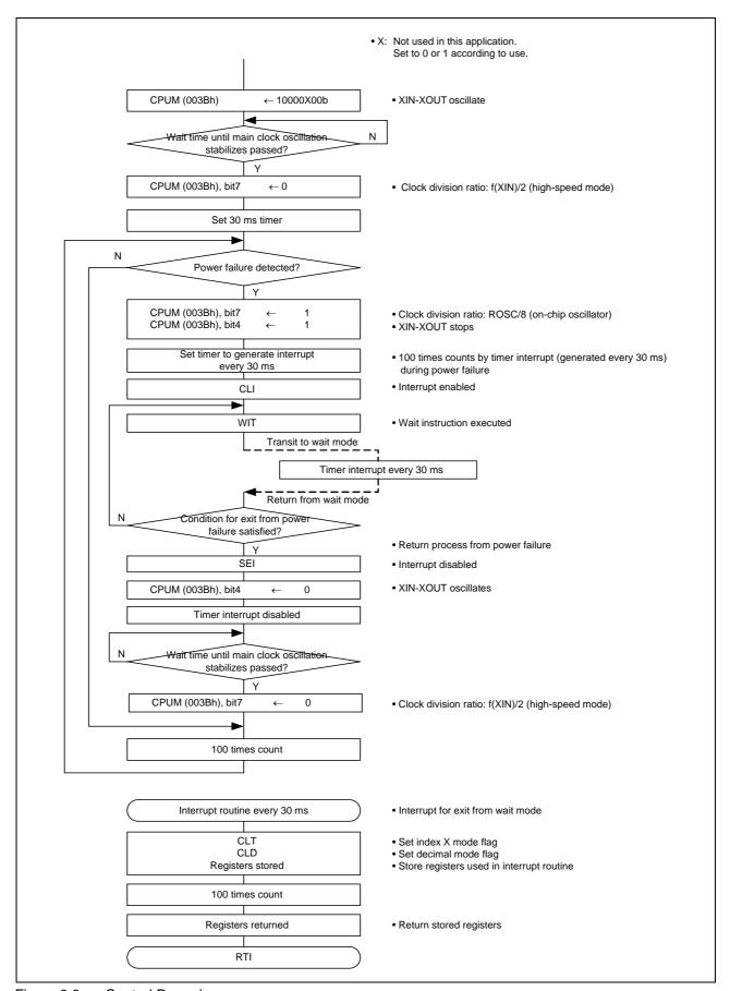
Figure 3.3 Control Procedure
