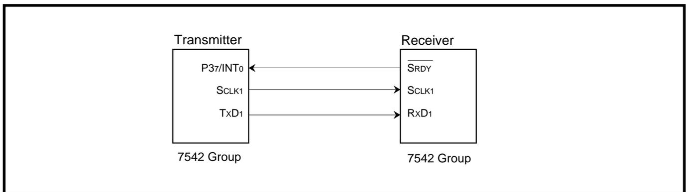
Figure 3 Connection diagram
