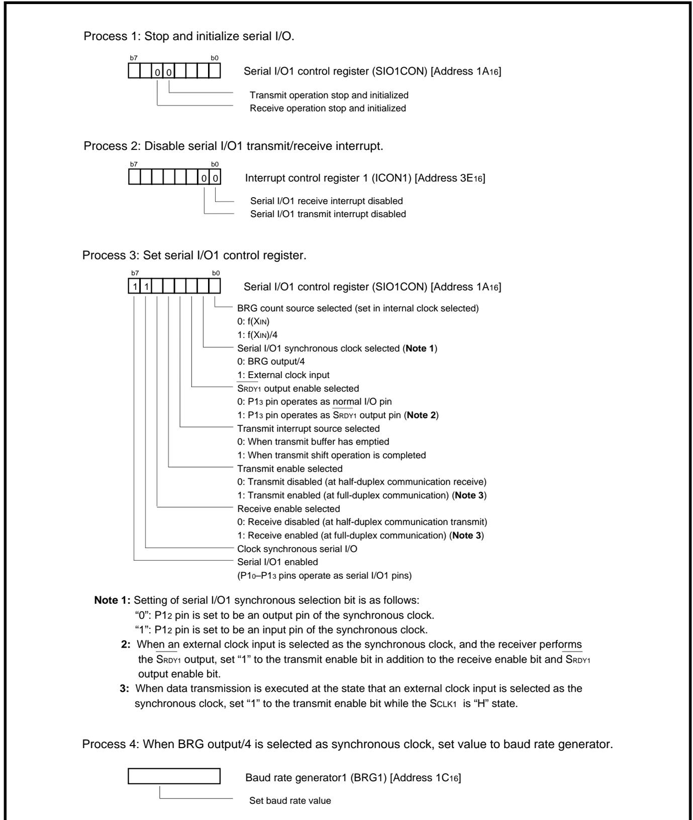
Figure 1 Setting method for clock synchronous serial I/O1 (1)
