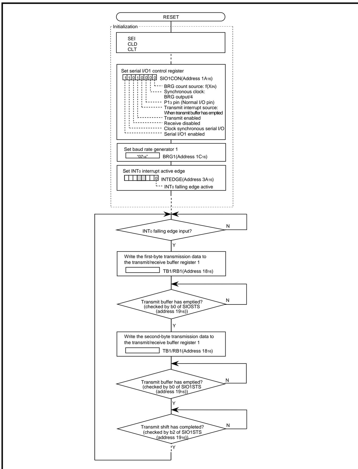
Figure 5 Control procedure of transmitter
