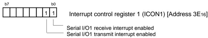
Process 7: Transmit/Receive of serial data (**Notes 1, 2**).
