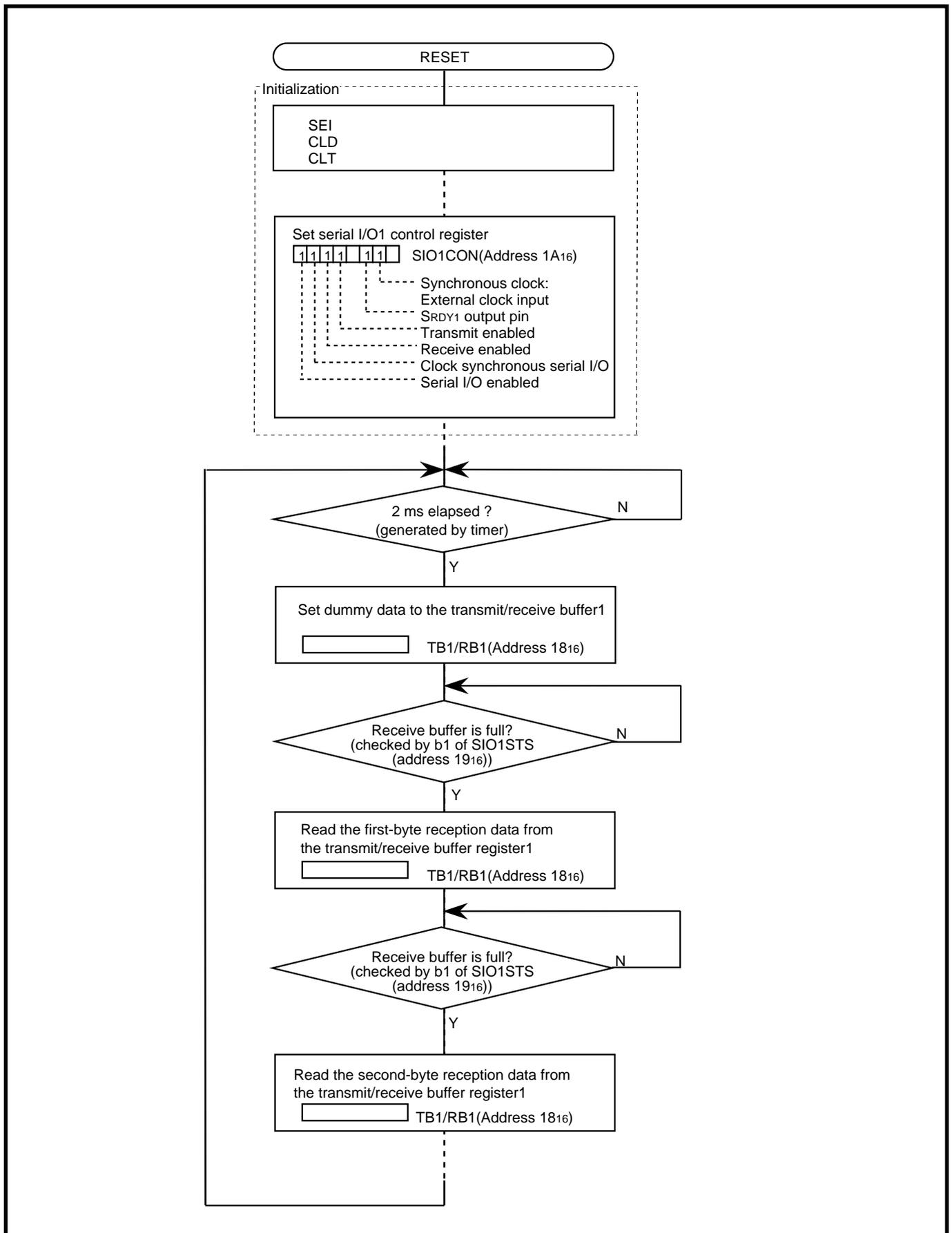
Figure 6 Control procedure of receiver
