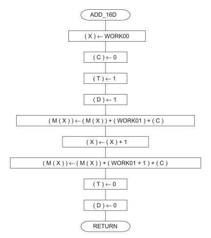
Note: M (X) represents the memory of the address indicated by Index Register X.
