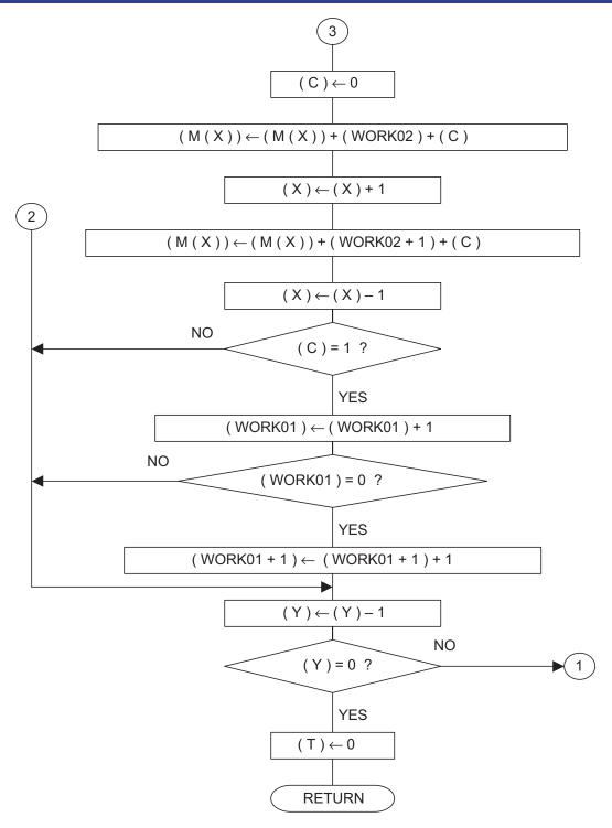
Note: M (X) represents the memory of the address indicated by Index Register X.
