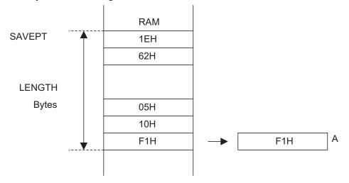
(b) Next, the memory contents of the next lower address are compared with the contents of Accumulator A. At this time, if the contents of Accumulator A are equal to or larger than the contents of the lower address, the contents of the memory and the Accumulator A are switched.
