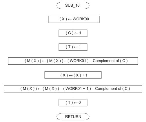
Note: M (X) represents the memory of the address indicated by Index Register X.
