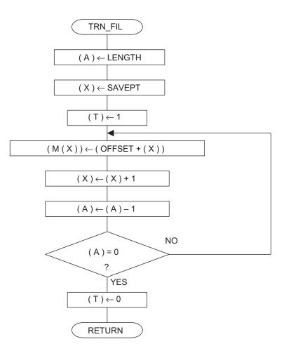
Note: M (X) represents the memory of the address indicated by Index Register X.
