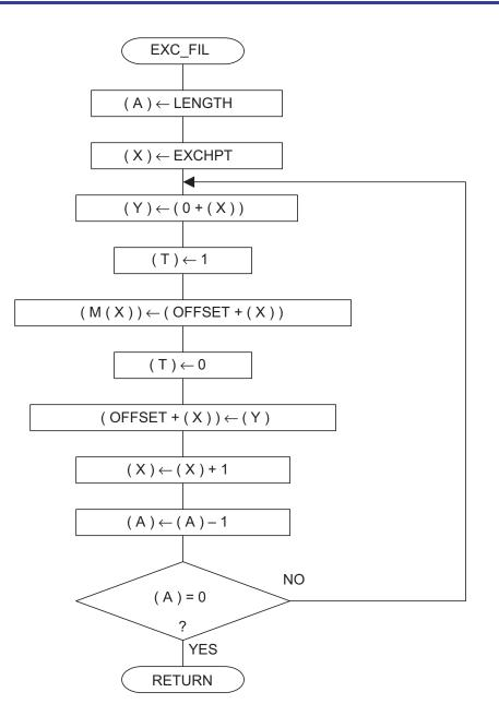
Note: M (X) represents the memory of the address indicated by Index Register X.
