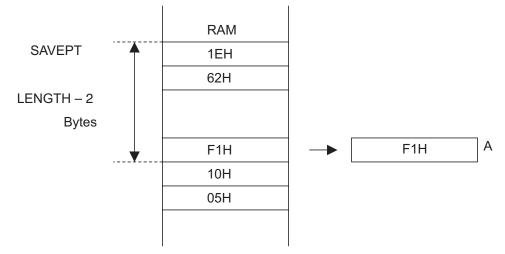
(g) In this manner, steps (a) through (d) are executed until the order of the contents is sorted into descending order, decreasing the highest address until it reaches the lowest address.
