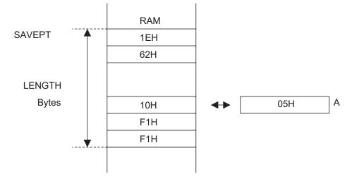
(d) This process is repeated until it reaches the lowest address and the contents of its memory are sorted, after which the lowest value will be stored in Accumulator A. The contents of this Accumulator A will be sent to the highest address in the memory.
