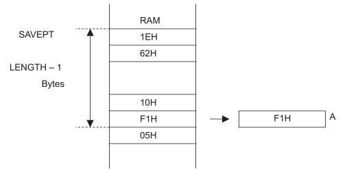
(f) Again, steps (a) through (d) are executed on the sorted area of which the highest address has been decreased, (LENGTH bytes - 2 bytes) from SAVEPT.
