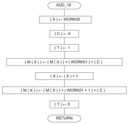
Note: M (X) represents the memory of the address indicated by Index Register X.
