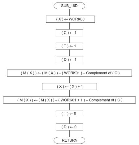
Note: M (X) represents the memory of the address indicated by Index Register X.
