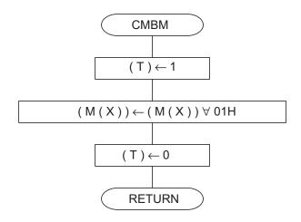
Note: M (X) represents the memory of the address indicated by Index Register X.
