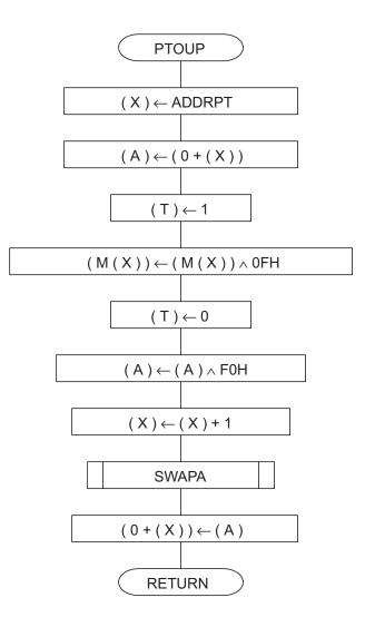
Note: M (X) represents the memory of the address indicated by Index Register X.
