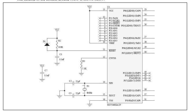
Figure 1 Schema of MCU Part
