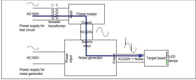
Figure 3 Diagram of Test Environment
