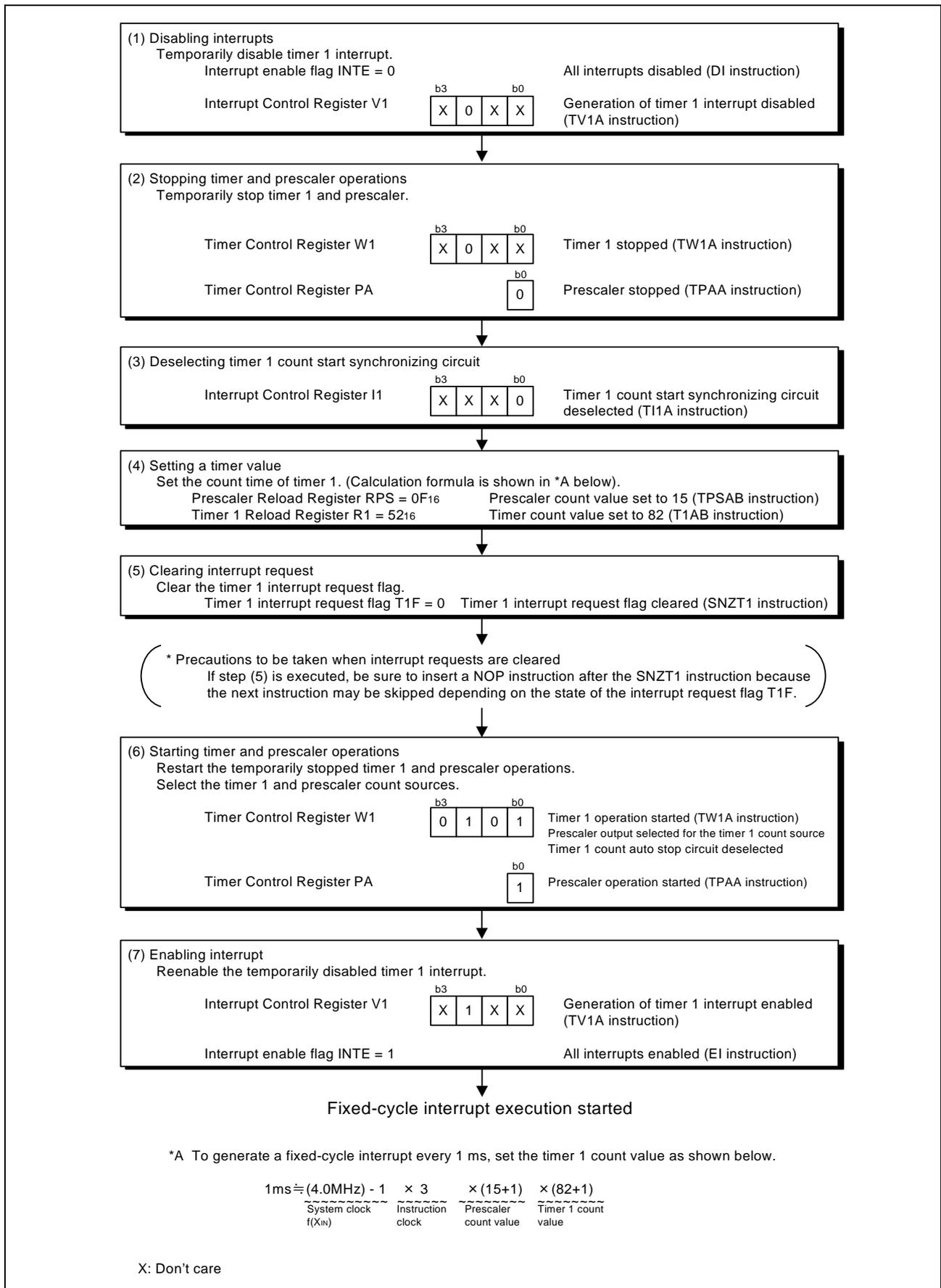
Figure 4.3 Example of Timer 1 Fixed-cycle Interrupt Setting
