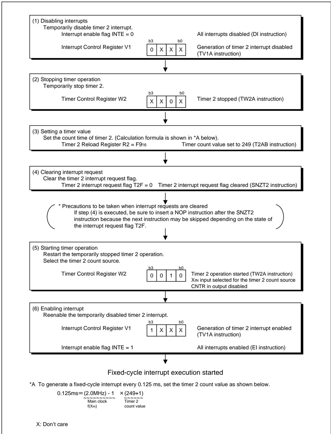
Figure 4.4 Example of Timer 2 Fixed-cycle Interrupt Setting
