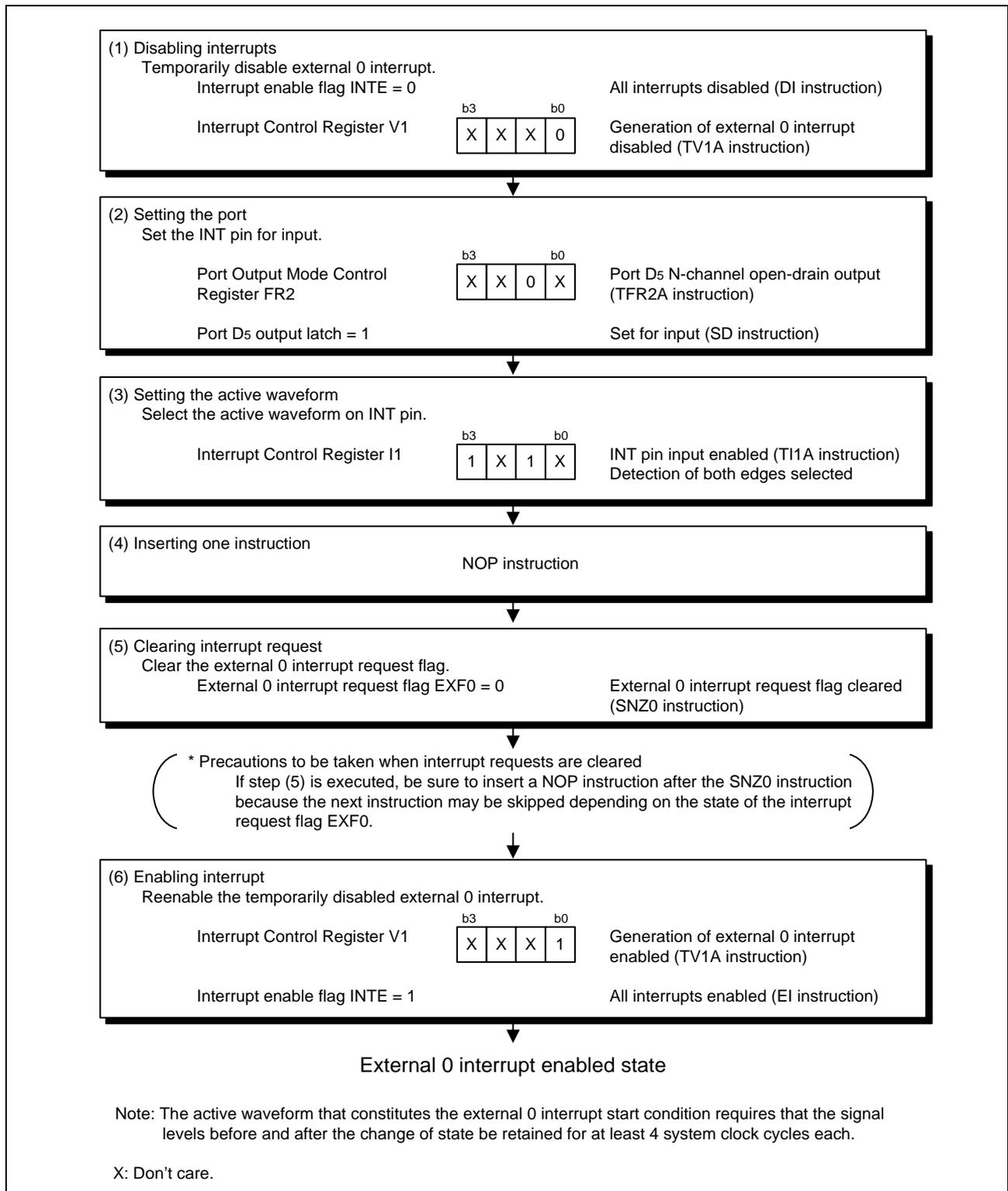
Figure 4.2 Example of External 0 Interrupt Setting
