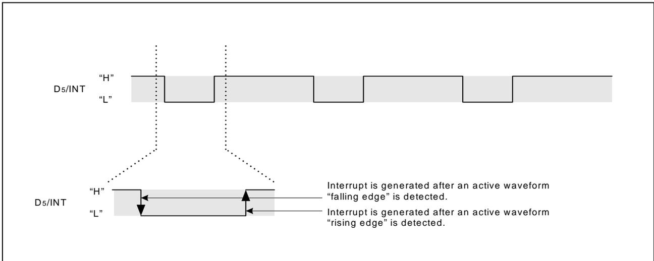
Figure 4.1 Example of External 0 Interrupt Operation
