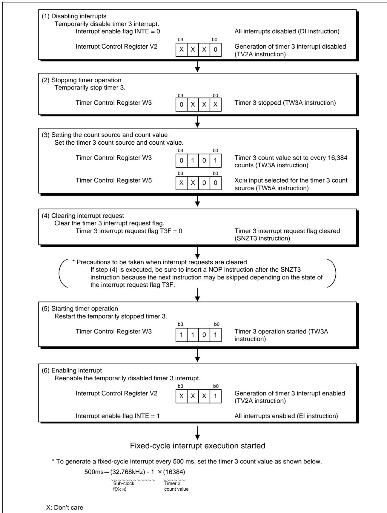
Figure 4.5 Example of Timer 3 Fixed-cycle Interrupt Setting
