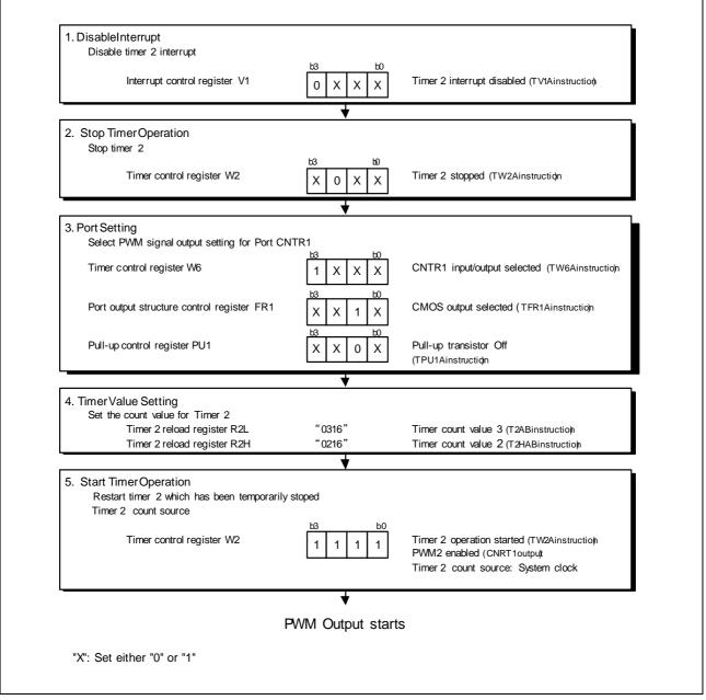
Figure 4.7 Setting Procedure for PWM Output Control
