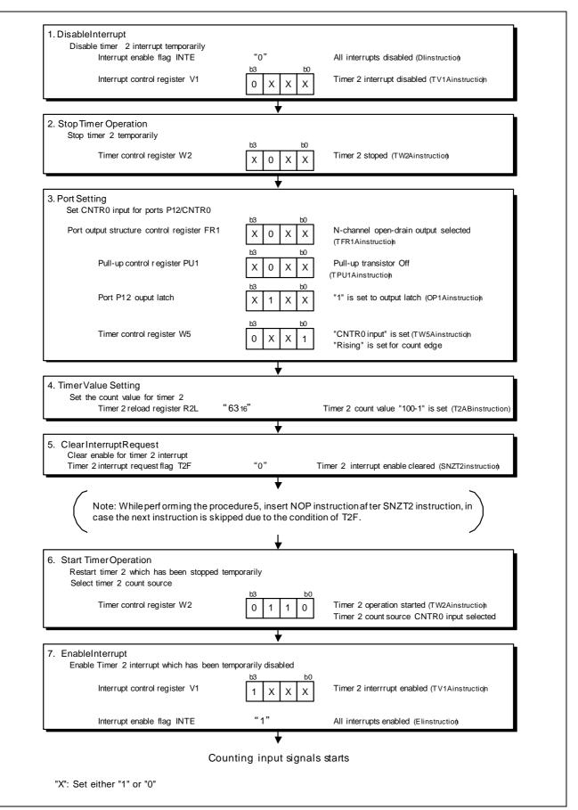
Figure 4.5 CNTR0 Input Setting Procedure
