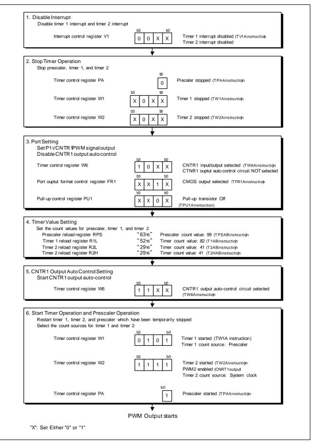
Figure 4.10 Setting Procedure for CNTR1 Output Auto-Control
