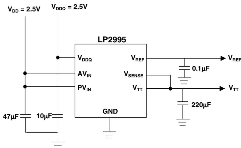
Figure 2. DDR Termination Regulator Scheme
