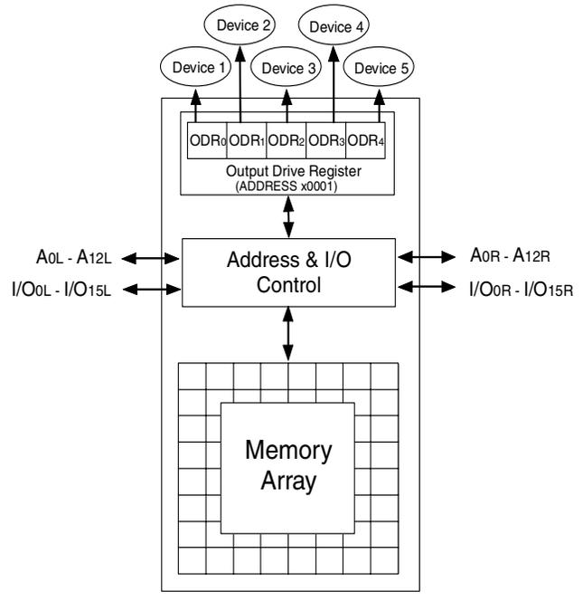
Figure 3. IDT70P248 Output Drive Register <sup>6482 drw 03</sup>
