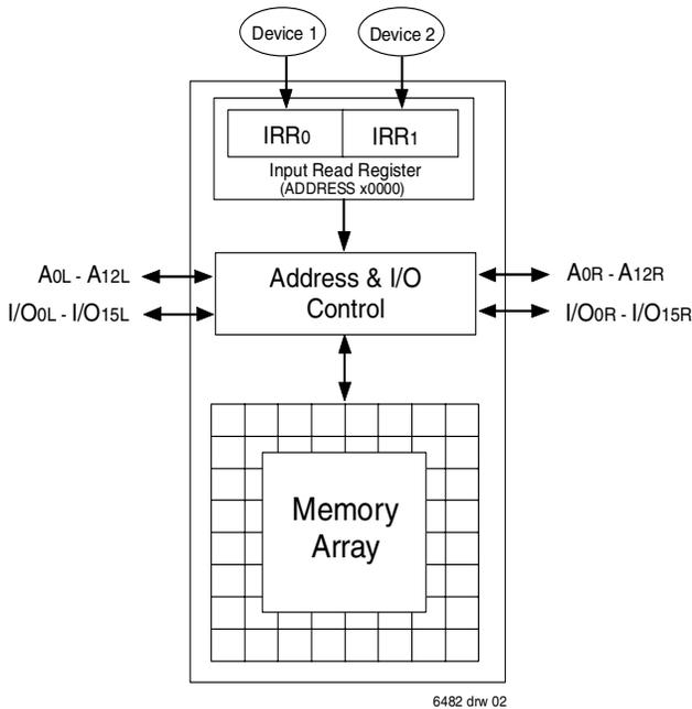
Figure 2. IDT70P248 Input Read Register <sup>6482 drw 02</sup>
