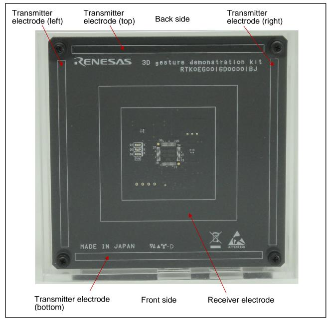
Figure 2-1 External Appearance (top view)
