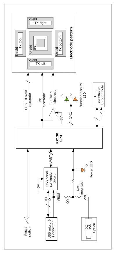
Figure 4-1 Block Diagram
