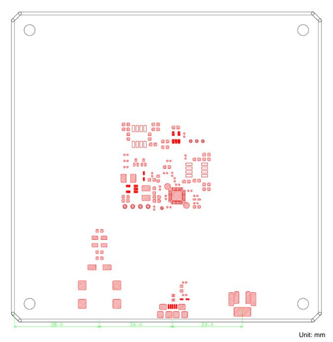
Figure 6-7 Solder Side Solder Mask
