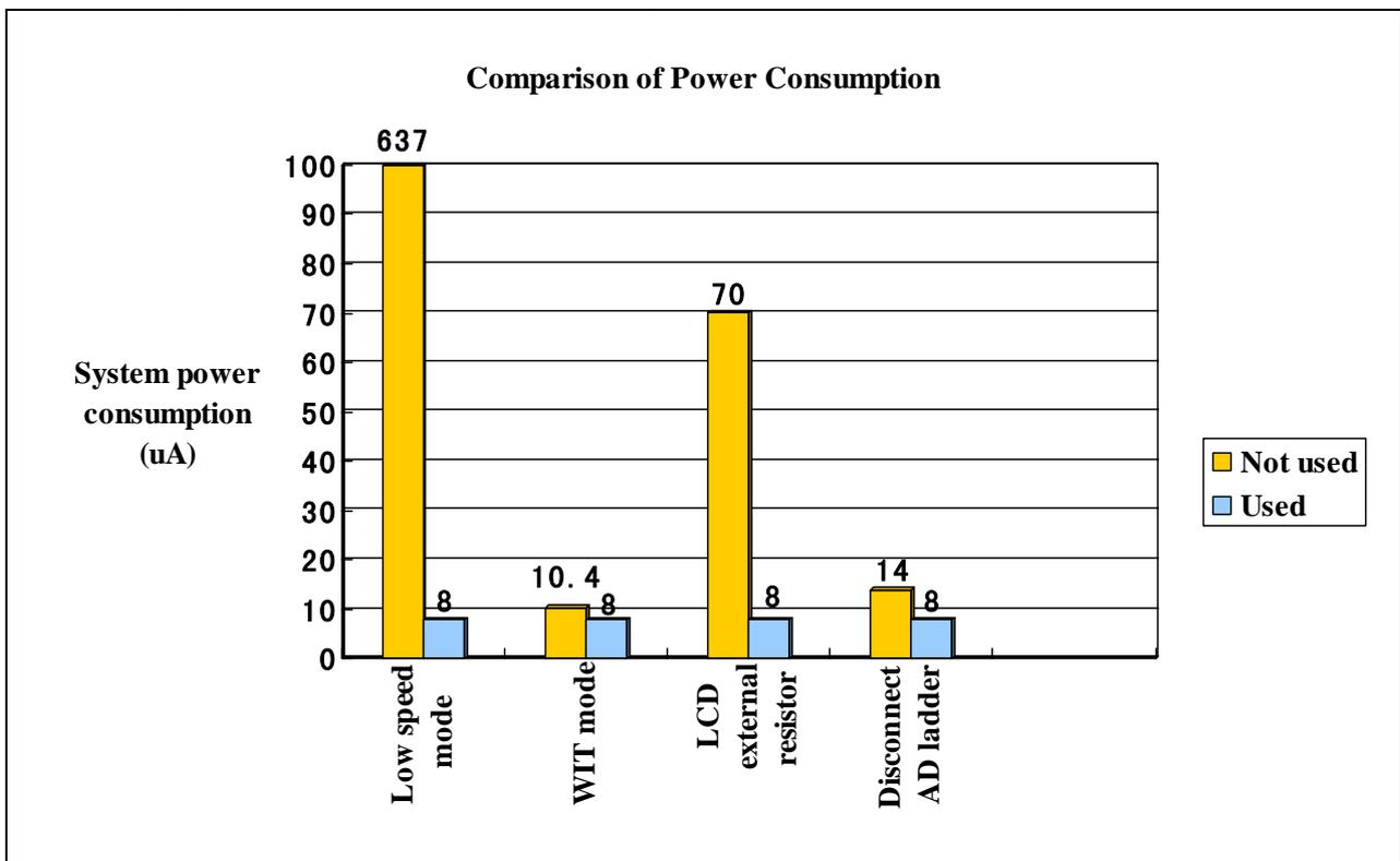
Figure 2 Comparison of System Power Consumption
