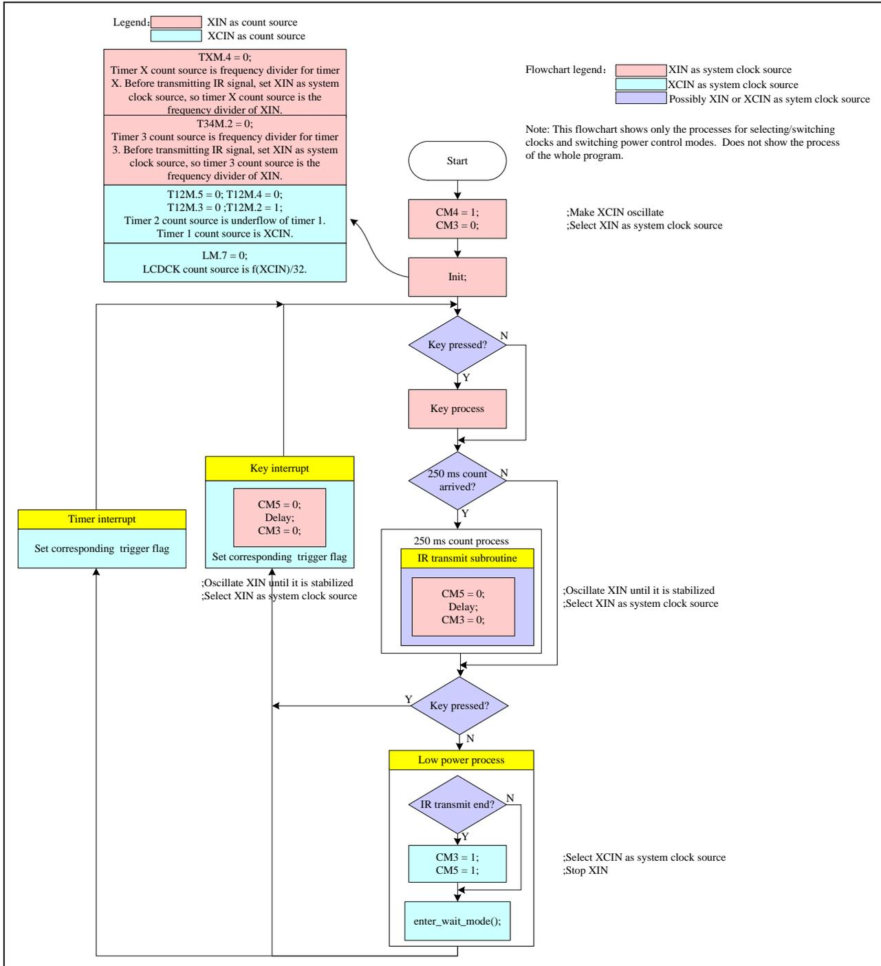
Figure 1 Flow Chart of Selecting/Switching Clocks in Work Mode
