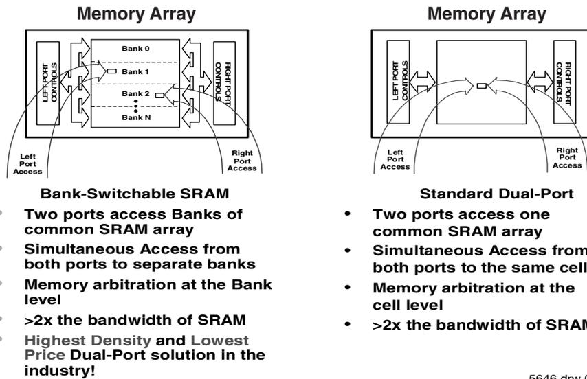
Figure 2. Comparison of BSDP and Standard Dual-Port
