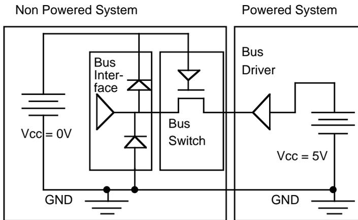
**Figure 5, Bus Switch on the Low Power Side**
