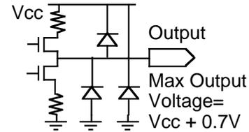
**Figure 3, An Output Structure Clamped to Vcc**
