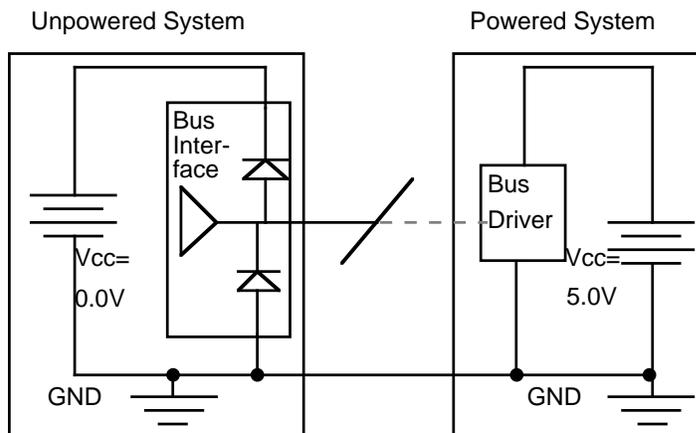
**Figure 4, Clamp diode on a 3-state bus**
