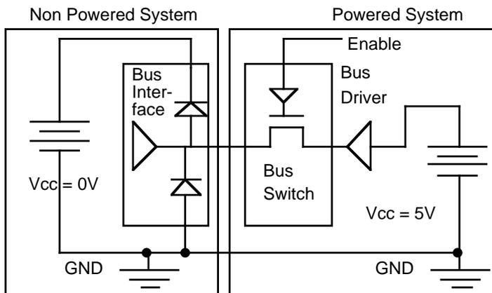
**Figure 6, Bus Switch on the High Power Side**
