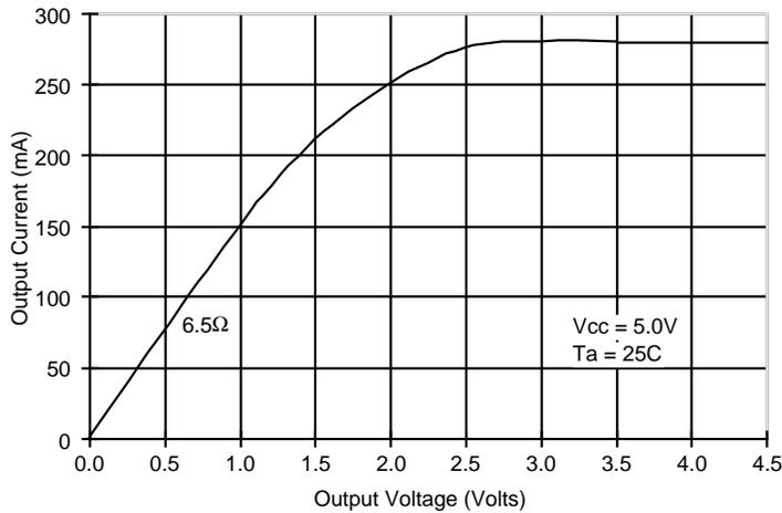
Figure 6, VOL Characteristics of High Drive
