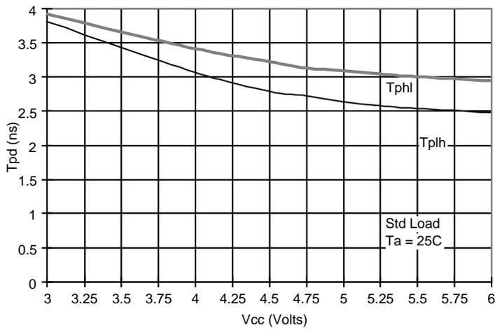
**Figure 21, Propagation Delay vs. Vcc (Balanced Drive)**
