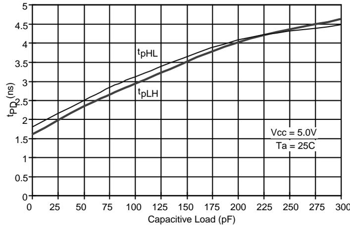
Figure 27, Delay vs. Load High Drive (FCT16244T example)
