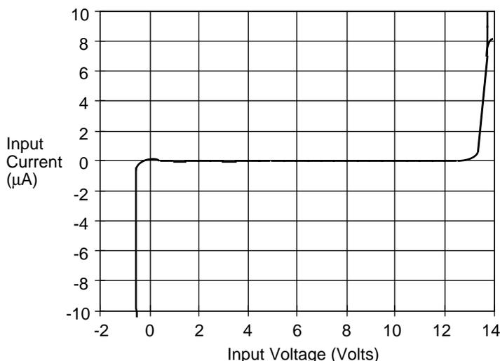
Figure 3, Input Impedance
