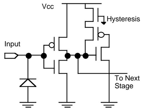
**Figure 1, Input Structure**
