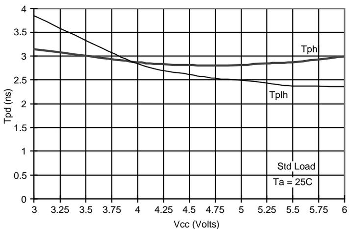
Figure 20, Tpd vs. Vcc (High Drive)
