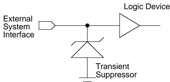
**Figure 9. Using a transient suppressor on a device input.**
