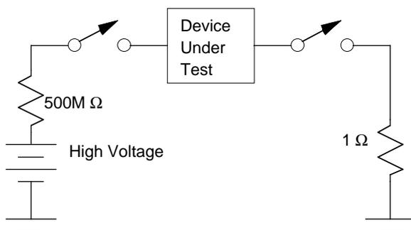
Figure 3. Charged Device Model for ESD testing.
