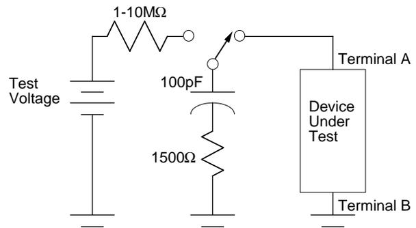
Figure 1. Human Body Model for ESD testing.
