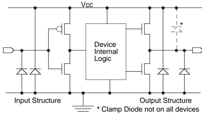
Figure 4. Clamp diode arrangement on IDT Logic Components.
