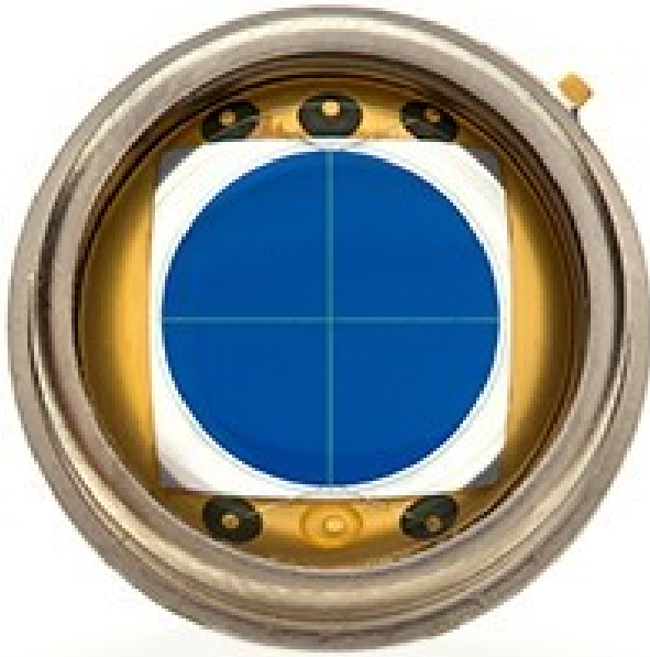
Figure 1. Photo of a quadrant photodiode with four matched photodiodes deposited on a single chip
