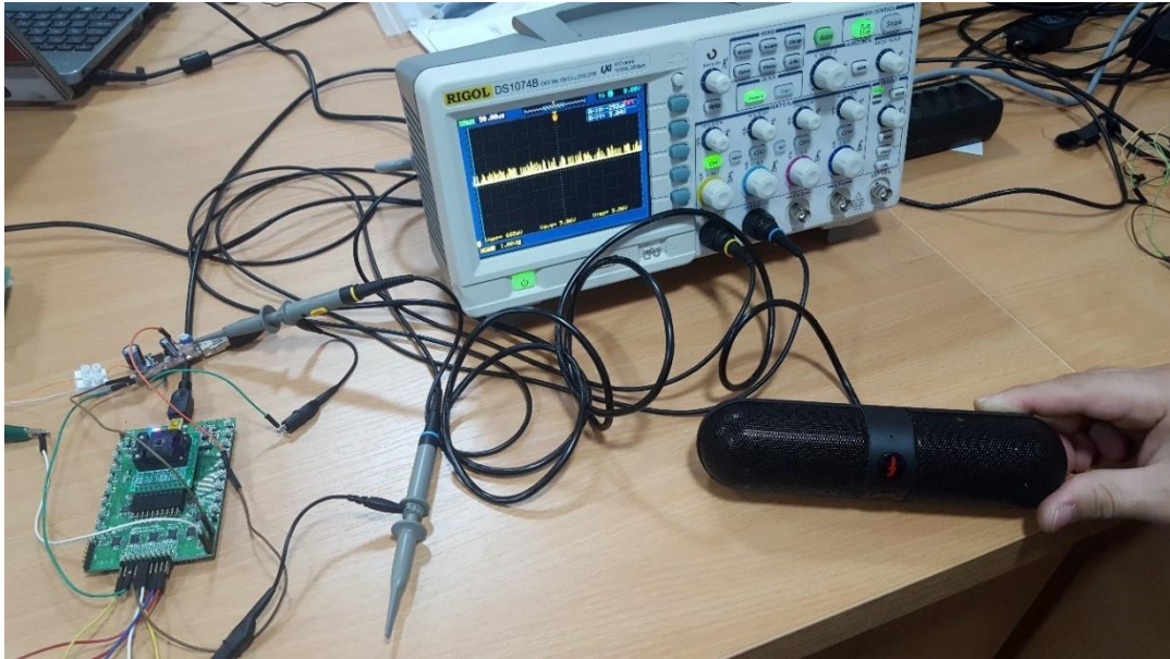
Figure 26. Boost implementation test charging Bluetooth speaker
