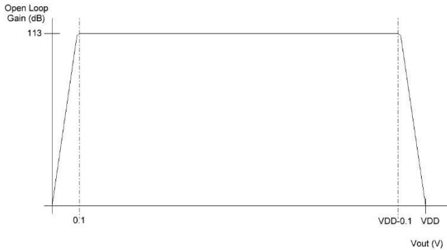
Figure 7. AOL vs VOUT Characteristics for SLG88102V
