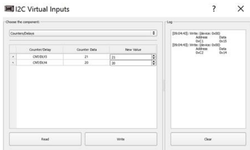
Figure 3(b). GreenPAK emulator I2C Virtual Inputs window
