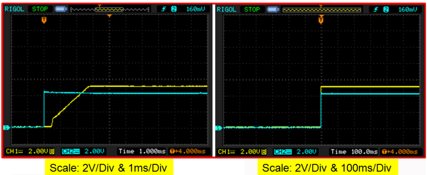
Figure 9. PowerMux Output Waveform for Condition#3
