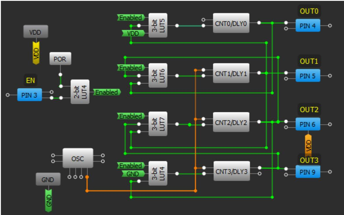
Figure 3. Power up and down sequencer block diagram
