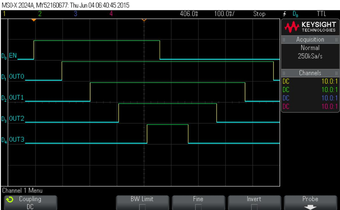
Figure 4. Power sequence up and down waveform
