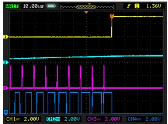
Figure 9. PWM generator turns off
