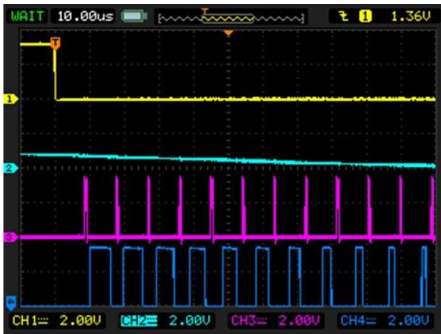
Figure 8. PWM generator turns on
