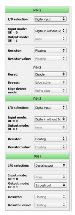
Figure 2. PINs configuration
