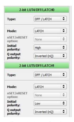
Figure 3. Latches configuration
