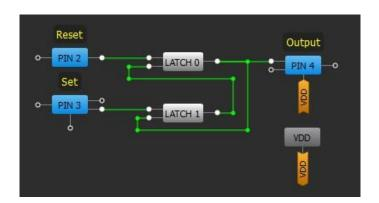
Figure 1. RS flip flop circuit design
