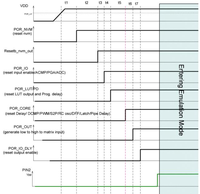
Figure 5. GreenPAK2 Startup
