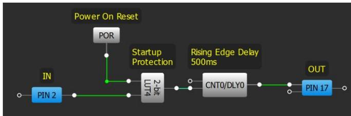
Figure 8. Circuit with Startup Logic
