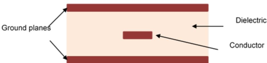
Stripline is another planar transmission line, consisting of a conducting layer and a pair of ground planes separated by dielectric.
