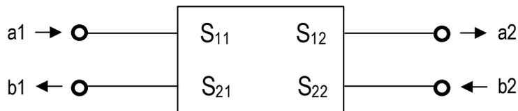
$S_{11}$  and  $S_{22}$  are the reflection coefficient, meaning the response at port 1 due to a signal at port 1 and the response at port 2 due to a signal at port 2.  $S_{12}$  and  $S_{21}$  are the transmission coefficient, meaning the response at port 1 due to a signal at port 2 and vice versa.
