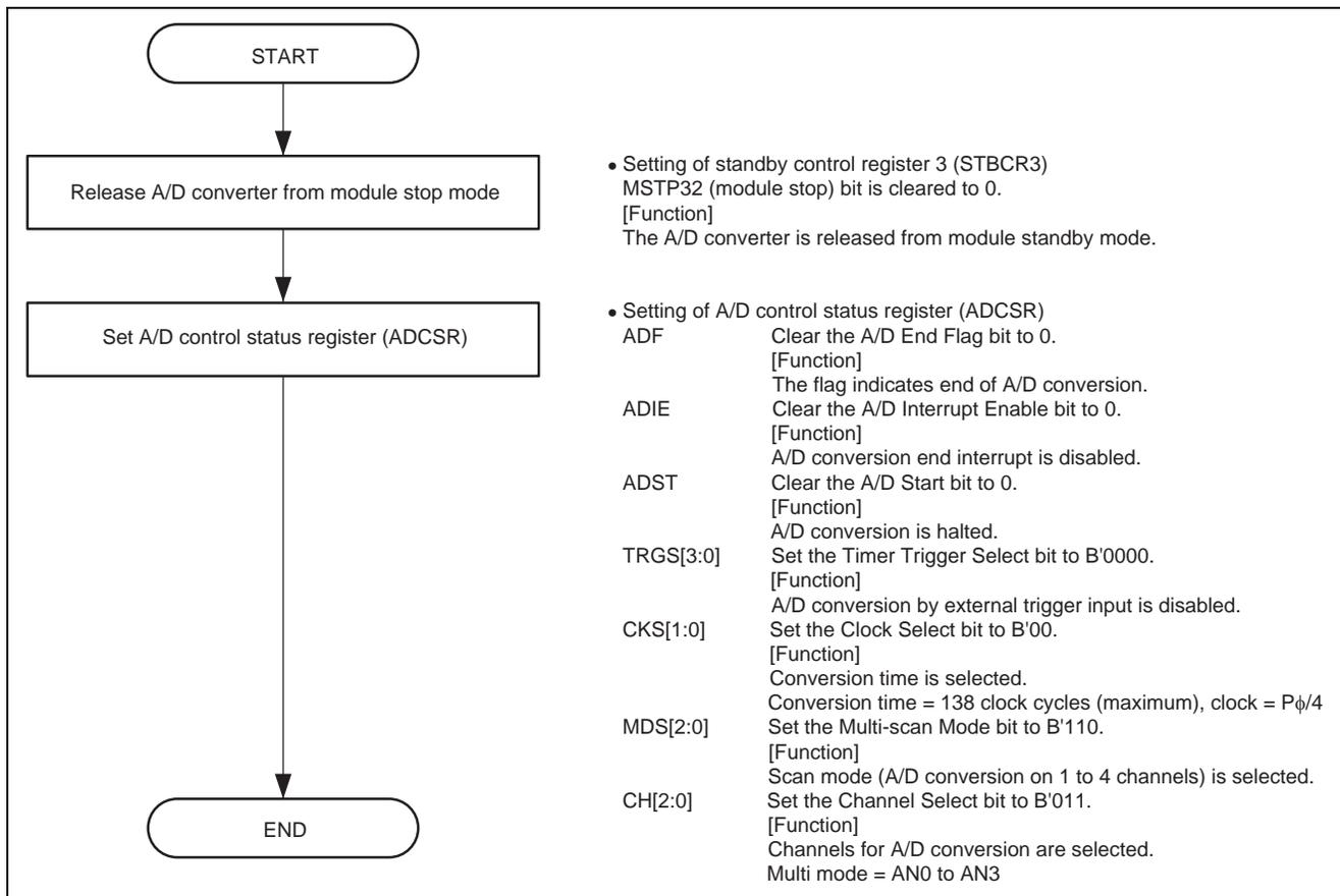
**Figure 2 Initialization Sequence for 10-Bit A/D Conversion**
