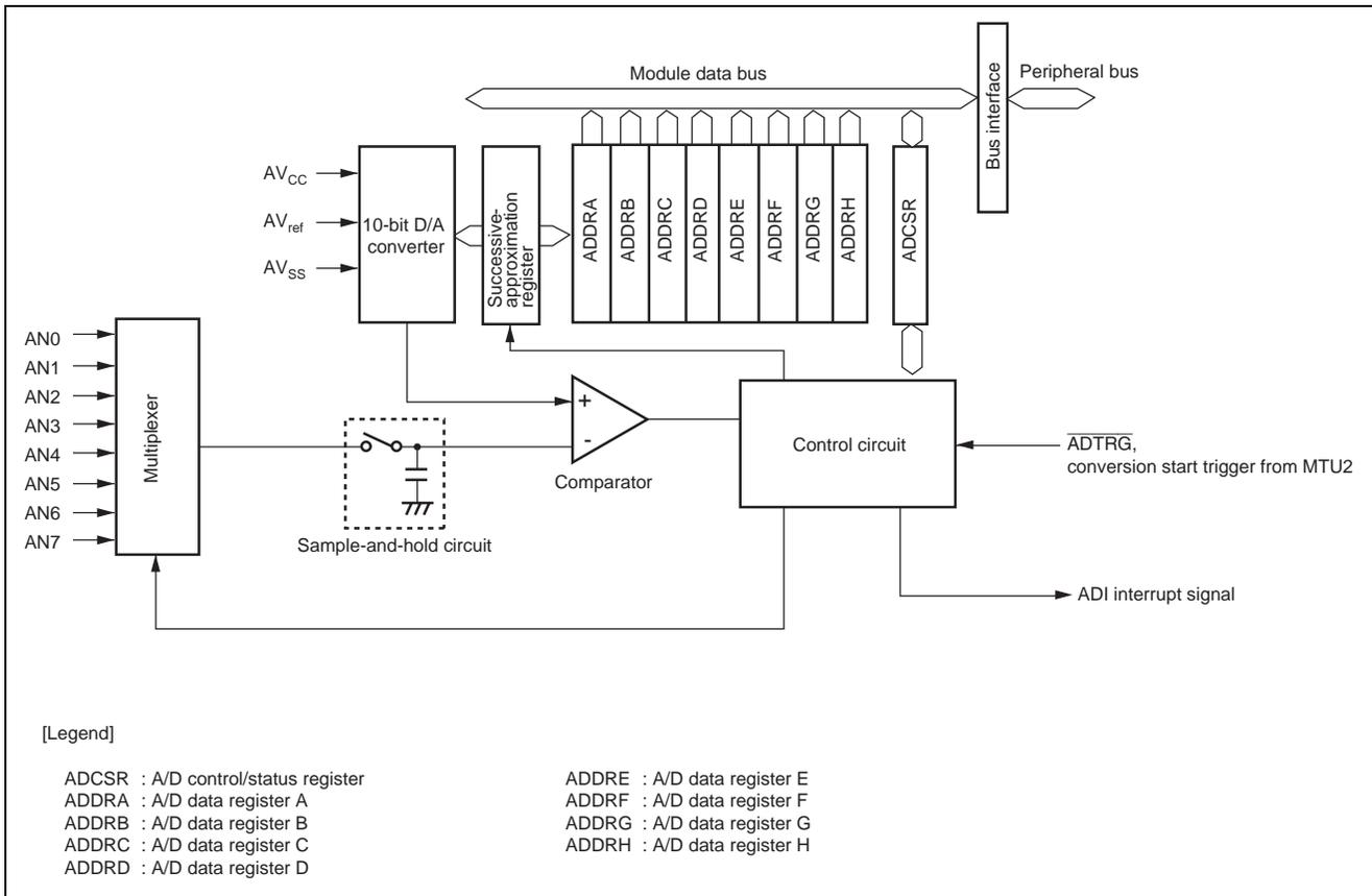
Figure 1 Block Diagram of the 10-Bit A/D Converter
