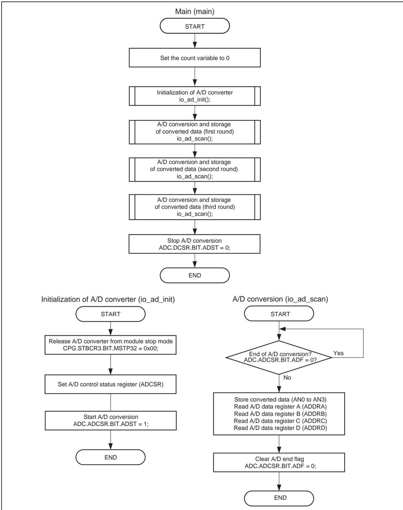
Figure 3 Flow of Handling the Sample Program
