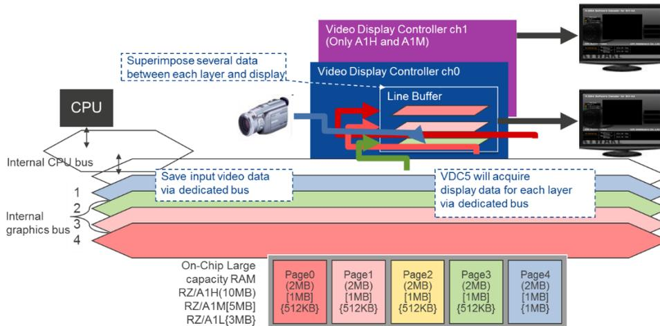
**Figure 9** Video and image subsystem of RZ/A1 MPUs
