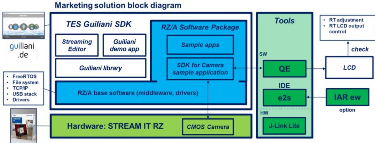
**Figure 4** RZ/A Software Package components and tools
