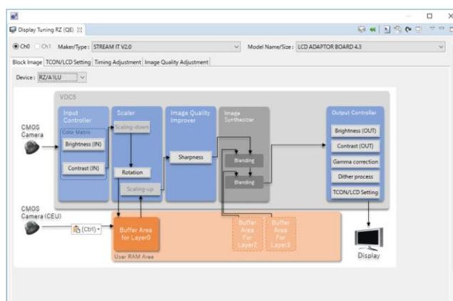
**Figure 10** VDC5-based image adjustments with QE Tool
